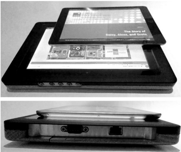
Fig. 1 Mobile computer designed by an SME following circular design principles compared to an iPad (fifth generation)
