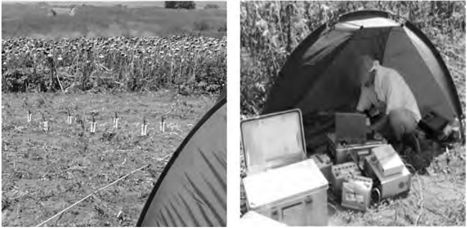
Fig. 5. Measurement set-up of a 3D-geoelectrical survey. At left: electrode array; at right: base unit with power supply
