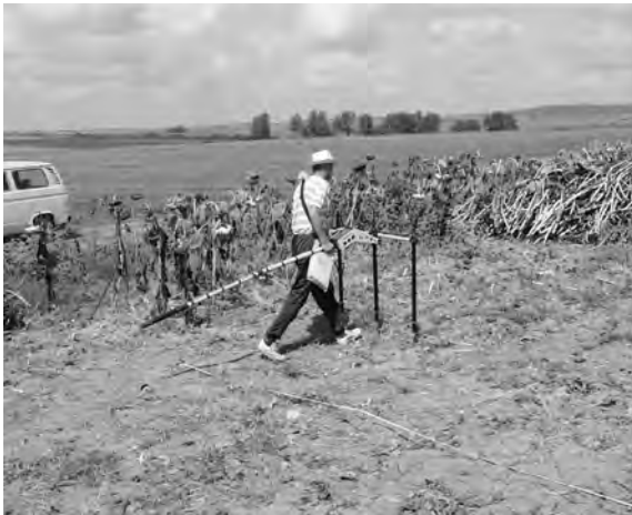
Fig. 1. The FEREX-magnetometer at work in Pliska
