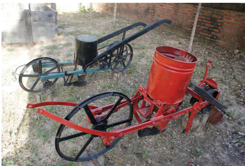
Figure 4.8 Mennonite seeders made from metal debris and oil canisters from the Chaco War in Colonia Menno (Source: author).
