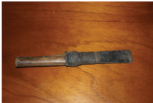
Figure 4.12 Ayoreo chisel made from Chaco War metal and telephone wire (Source: author).
