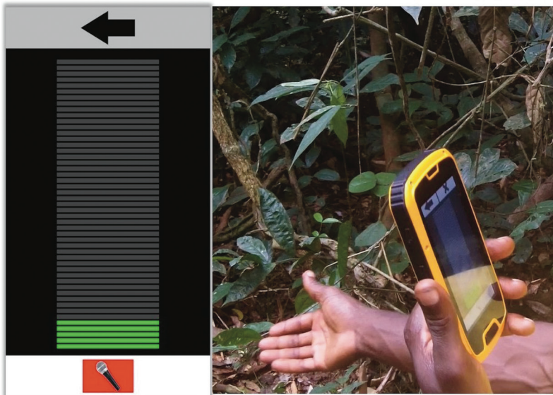
Fig. 12.2 A red indicator to show when audio recording is ongoing helped to reduce confusion and mistakes by participants. Credit: Photograph taken by Simon Hoyte 2017 (right); Sapelli platform UCL Extreme Citizen Science research group (ExCiteS; left).
