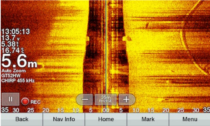
Figure 20.16: Side-scan sonar image of a pipeline. Photo: Samir Bhowmik.
