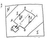
Luttent is going through the contractor through the Coil frows A on B. The force according to Die Right-hand-Stape rate will be down on side AB and up on side PC. This causes a net image cond solution anti-clockwesse.
