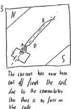
3. The current has now been cut off from the coil due to the commutator thus there is no force on the coils.
