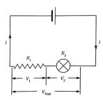
FIGURE 4.1.7 Using Ohm's law, it is possible to show the relationship between the potential difference supplied by the cell, V<sub>fotal</sub>, the current flowing in the circuit, *I*, and the resistances of the two components *R*<sub>1</sub> and *R*<sub>2</sub>.
