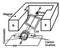
Explain the sequence of events that occur with the commutator, and the current and force, to keep the motor spinning. Draw simple diagrams to illustrate your explanation.
