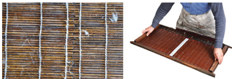
Fig. 5c: Laid paper made with the mould equipped with the bamboo sieve. Figs 5a–c: Photographs by Agnieszka Helman-Ważny, diagrams by Dorota Helman.
