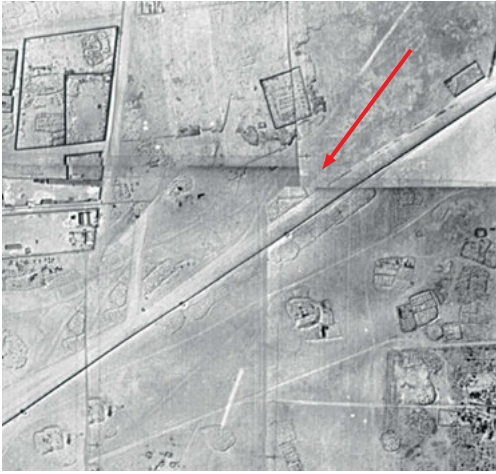
3.4 Detail of the 1951 photomosaic of aerial photographs of Kuwait with arrow indicating the edge of overlapping photographs.
