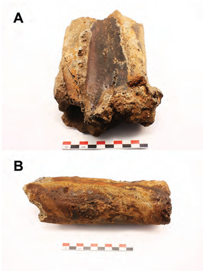
FIGURE 5.6 Multiple fused tuyeres (A). Single tuyere (B)
