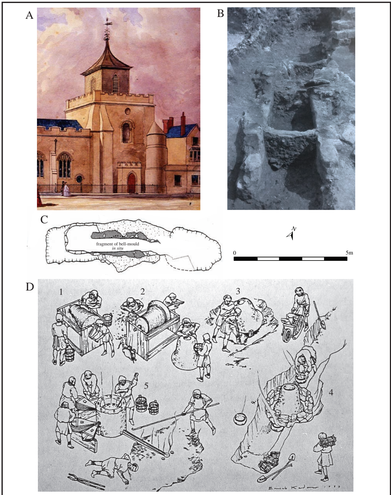
Fig. 7.18 The bell-casting pit in Mary Major church. (A) The tower in which the pit was found (© Devon and Exeter Institution). (B) View of the pit from the south-west. (C) Plan. (D) Reconstruction of the bell-founding process. Upper: forming the core; forming the wax model; lowering the assembled moulds into the pit. Lower left: casting the bell. The bell-founder listens to the ground as metal runs from the furnace into the casting pit and labourers work the bellows (B–D Exeter Archaeology archive; © Exeter City Council; (D) drawn by Erich Kadow, based on interpretation of Theophilus by C.G. Henderson)
