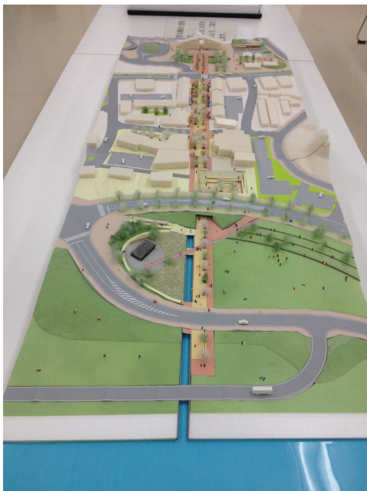
Figure 12.6 Onagawa town model illustrating the spatial and sectional relationship to the waterfront from the town center and coastal highway. Note the top of the model is the new train station with the main street to the water passing under the coastal highway with a flood gate positioned to close in case of disturbance. Image Credit: Azaroff.
