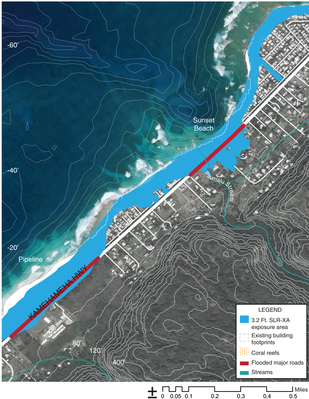
Figure 10.4 Sunset Beach map shows the projected 3.2-foot SLR-XA area (in light blue), including flooded stretches of the coastal road (in red). Image courtesy of PaclOOS.
