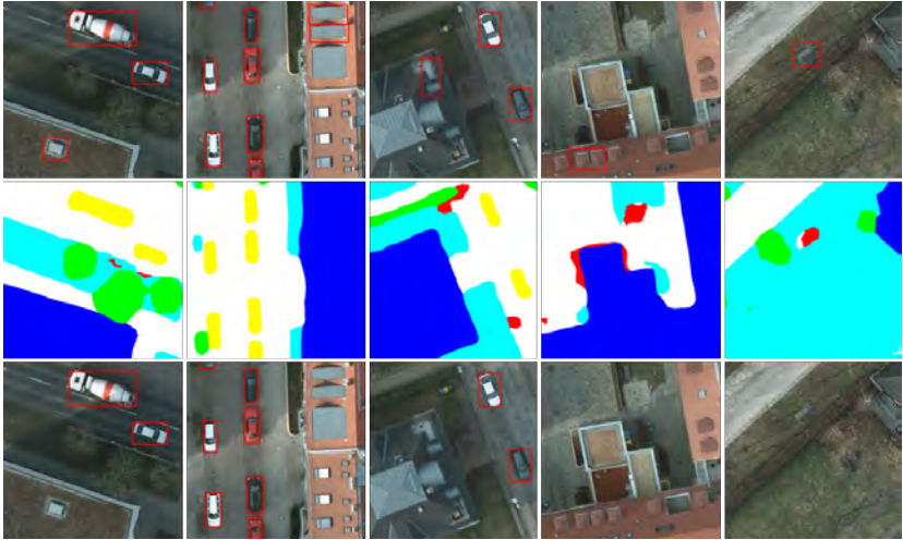
Figure 6.12: Qualitative detection examples before (top row) and after (bottom row) filtering the region proposals using the semantic labeling mask outputted by FCN-D16 indicate that false alarms located on regions that are unlikely to contain vehicles, e.g., windows on buildings, are removed.
