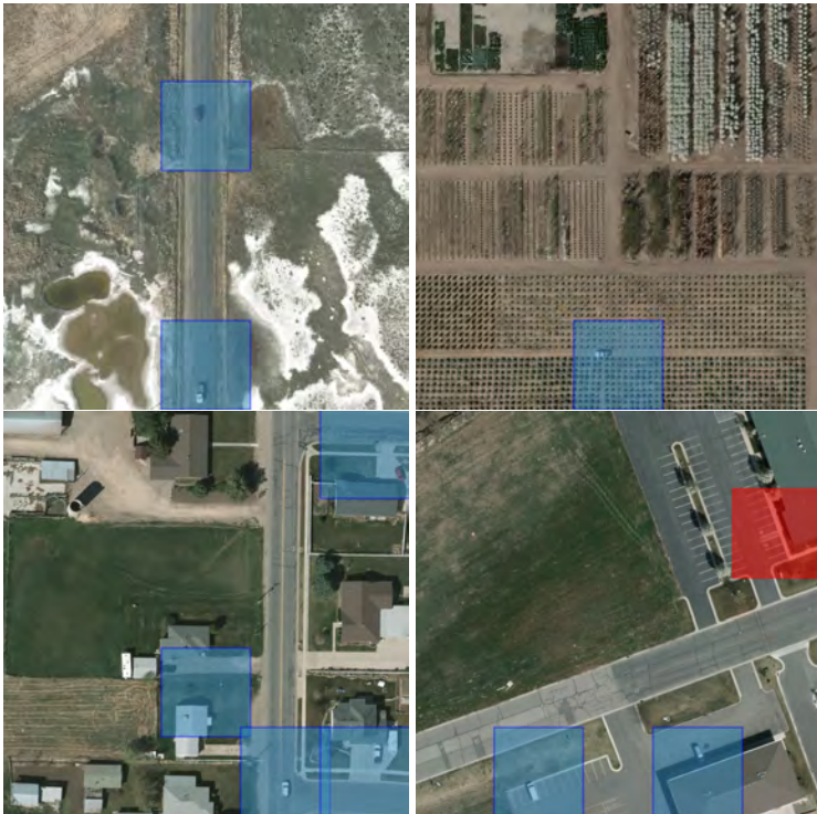
Figure 7.10: Classification results of the SAR module on VEDAI. Highlighted regions are classified as region with at least one object and are considered for detection. Regions labeled in blue contain vehicles, whereas regions labeled in red contain no vehicles.
