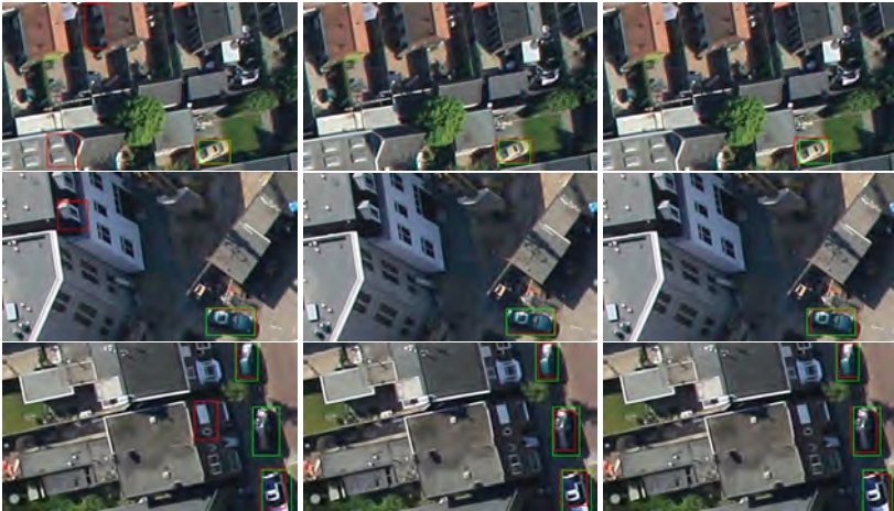
Figure 8.8: Qualitative detection results (red boxes) and corresponding GT (green boxes) for Faster R-CNN with VGG16 (left column), EMT-MFD Faster R-CNN with VGG16 (middle column) and EMT-MFD Faster R-CNN with ZynqNet (right column) on the ITCVD dataset demonstrate that the proposed approaches are more robust to false alarms due to vehicle-like structures in unseen data, while vehicles are correctly detected.
