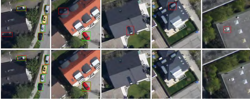
Figure 6.21: Qualitative detection examples of the baseline Faster R-CNN (top row) and EMT Faster R-CNN with FCN-D16 (bottom row) indicate that false alarms located on regions that are unlikely to contain vehicles, e.g., buildings, are reduced.
