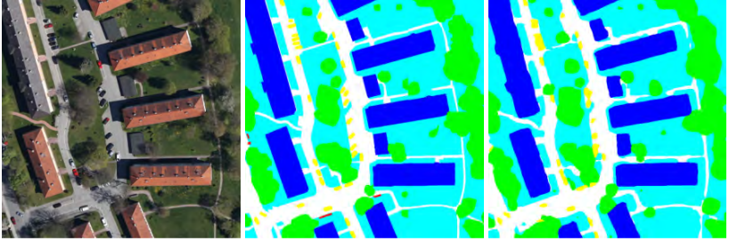
Figure 6.19: Qualitative semantic labeling results of FCN-D16 (left column) on DLR 3K and corresponding GT (middle column) indicate limitations of the employed semantic labeling architecture in case of tiny structures such as vehicles, i.e., inaccurate boundaries.
