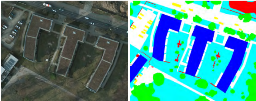
Figure 4.6: Example patch of the Potsdam dataset (left) and the corresponding semantic labeling mask (right) with pixel-wise semantic annotations of six categories: impervious surface (white), building (blue), low vegetation (cyan), tree (green), car (yellow), and clutter (red).
