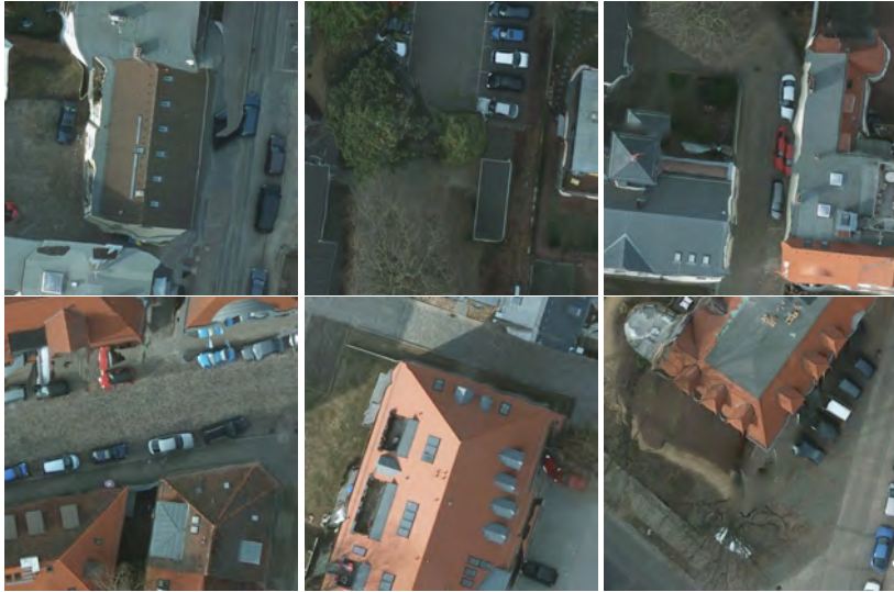
Figure 6.17: Artifacts of the RGB images of the Potsdam dataset due to ortho-rectification.
