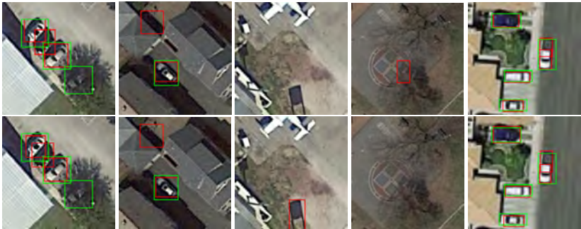
Figure 8.12: Qualitative examples of missed detections and false alarms for EMT-MFD Faster R-CNN with VGG16 (top row) and ZynqNet (bottom row) on the DOTA dataset. Missed detections are mainly due to objects that are partially occluded, e.g., by trees, while false alarms are mostly caused by shadows or structures located on asphalted areas. Furthermore, false alarms are caused by split detections due to vehicle types that are not represented in the training data.
