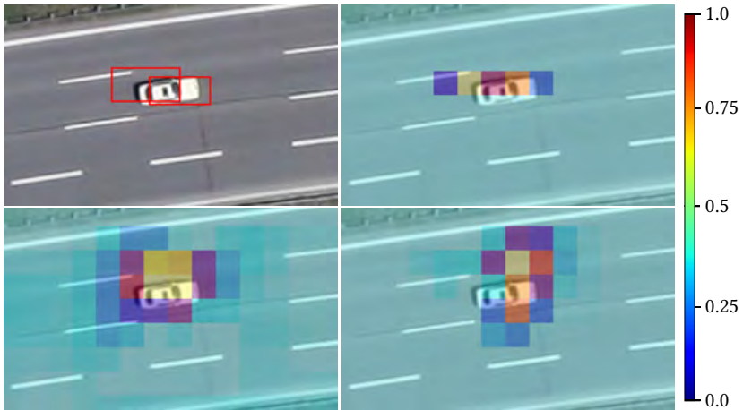
Figure 5.5: Activations of three filters from conv5_3 used as feature map and the corresponding detection results indicate that the feature map resolution is not sufficient to accurately localize small objects as in case of DLR 3K. The activations are normalized to values between 0 and 1.
