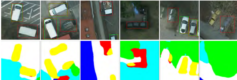
Figure 6.16: Qualitative examples of remaining FPs for EMT Faster R-CNN with FCN-D16. Most FPs can be attributed to vehicle-like structures positioned near roads or beneath trees, while almost no FPs on buildings remain.
