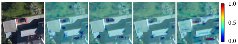
Figure 5.21: Activations of four filters from conv3_3 that respond to particular vehicle parts but also to similar structures.
