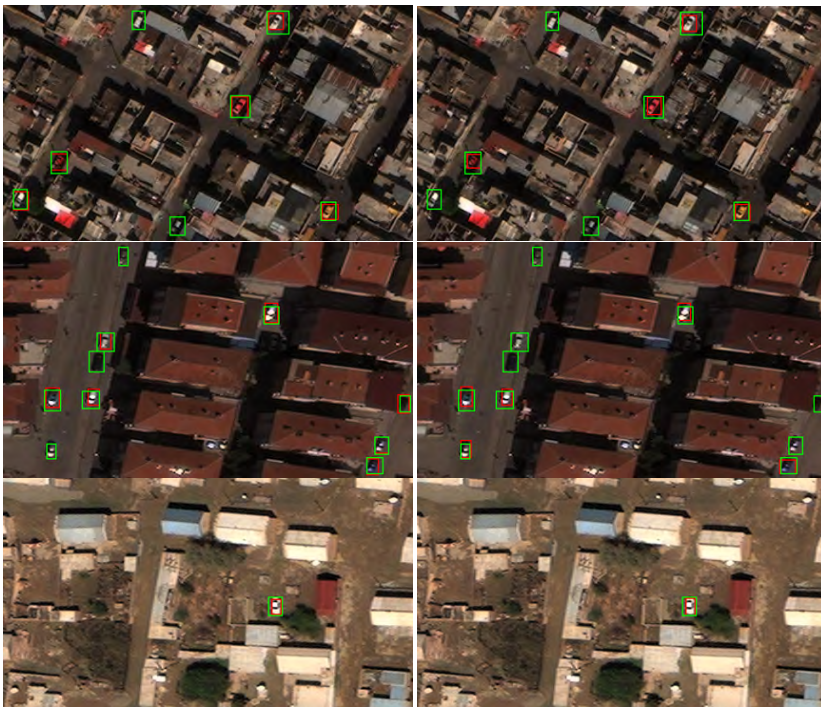
Figure 8.13: Qualitative detection results (red boxes) and corresponding GT (green boxes) for EMT-MFD Faster R-CNN with VGG16 (left column) and with ZynqNet (right column) on the xView dataset. Despite the low spatial resolution, the proposed approaches are robust to false alarms due to vehicle-like structures in unseen data with differing scenarios and backgrounds. However, multiple missed detections occur due to the relatively large differences to the training data.
