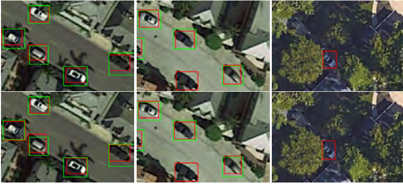
Figure 8.10: Qualitative detection results (red boxes) and corresponding GT (green boxes) for EMT-MFD Faster R-CNN with VGG16 (top row) and with ZynqNet (bottom row) on the DOTA dataset indicate the good detection accuracy in unseen images from different sensors. Note that even vehicles with missing annotations are detected.
