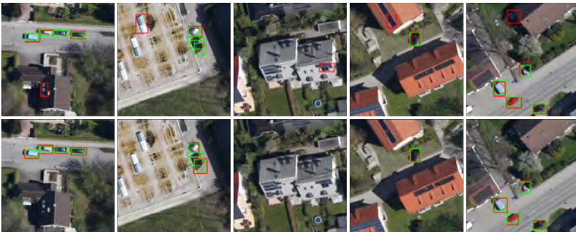
Figure 6.3: Qualitative detection (red boxes) and corresponding GT (green boxes) for Faster R-CNN using conv3_3 as feature map (top row) and MFD Faster R-CNN (bottom row) for a GSD of 26 cm. The number of FPs due to objects with shapes similar to vehicles are reduced by integrating spatial context information from deeper layers.
