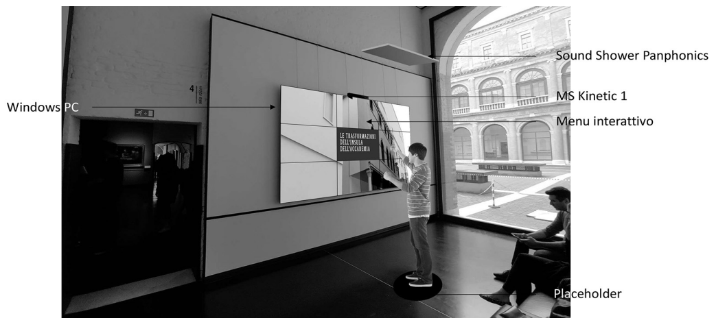
Fig. 2. Devices of the new interactive installation.
