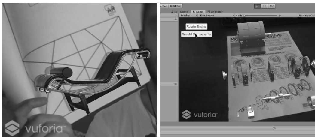
Fig. 2. AR exercises based on image tracking, developed in Unity and Vuforia. On the left: the object is superimposed against its design drawing. On the right: the user can start an animation to see the engine model disassembled; the figure shows the app preview in the Unity development interface. Authors: M. Ferraro, M. Marangone, D. Parente (left) E. Burati, A.L. Scardino, M.A. Valencia Zeballos (right).
