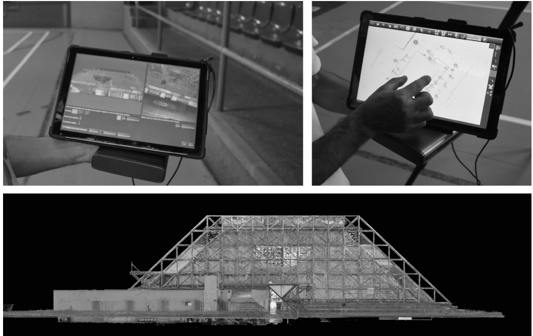
Fig. 4. Positioning of the laser scanner and its point cloud in the Sport Hall.
