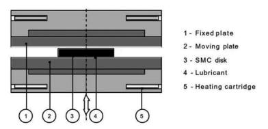
Figure 2-6: Schematic illustration of the simple compression rheometer. To gain simple compression, the mold surfaces are lubricated [Dum03]
