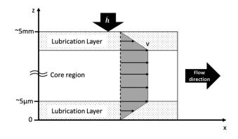
Figure 3-22: Schematically cross-Section of SMC material during the molding process
