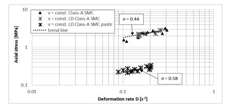
Figure 3-12: Fitting of the viscosity power-law exponent n with the results for the constant closing speed ( $\dot{h}$  = 1 mm s<sup>-1</sup>) of the Class-A, LD Class-A SMC and the LD Class-A SMC paste
