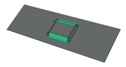
Figure 4-23: IRTG reference structure with the position of the local reinforcements (green)
