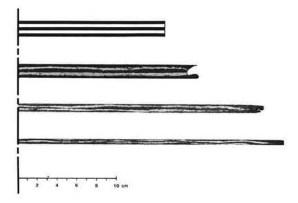
Figure 2-4: Experimental investigation of the flow behavior of SMC by using differently colored SMC sheets [Bar85]
