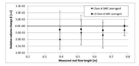
Figure 3-10: Averaged relative volume change  $\beta$  from the Class-A SMCs experiments for a constant closing speed of  $\dot{h} = 1 \text{ mm s}^{-1}$
