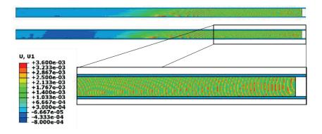
Figure 4-21: Comparison of the displacement in flow direction (U1) of the carbon UPPH SMC (top) and VE SMC (bottom) after 0.025 s simulation time
