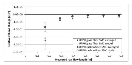
Figure 3-11: Relative volume change  $\beta$  from the experiments of the glass and carbon UPPH SMC for a nominal deformation rate of D = 0.25 s<sup>-1</sup>
