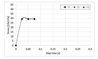
Figure 4-17: Simulated stress distribution for Sensor 1 to 3 for the Class-A-SMC material
