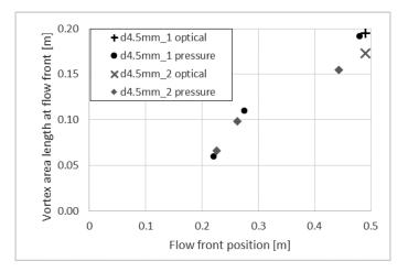
Figure 3-19: Length of the vortex area at the flow front: optical measured and extracted from pressure distribution
