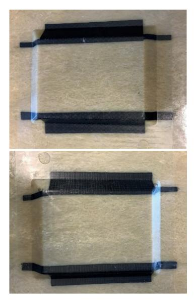
Figure 4-26: Photos of the molded reference structure with local reinforcements with no deformation of the tapes (top) and slide deformation at the end of the tapes (bottom) [But17]
