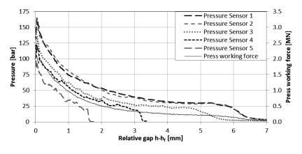
Figure 3-4: Exemplary pressure distribution of the LD Class-A SMC for a closing speed of  $\dot{h} = 1 \text{ mm s}^{-1}$  [Hoh17b]
