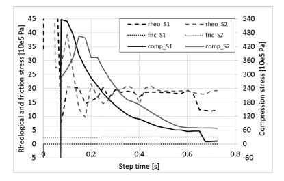
Figure 4-15: Rheological, friction and compression pressure stress for a VE-SMC material formulation at sensor position 1 and 2
