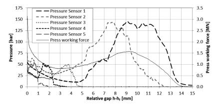
Figure 3-6: Exemplary pressure distribution of the UPPH glass fiber SMC for a closing speed of  $\dot{h} = 1 \text{ mm s}^{-1}$
