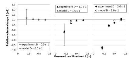
Figure 3-9: Comparison of the relative volume change  $\beta$  of the VE-SMC between measurement and modelling for three nominal deformation rates D = 0.5 s<sup>-1</sup>, 1.0 s<sup>-1</sup> and 2.0 s<sup>-1</sup> during the molding process [Hoh17a]
