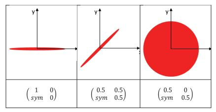
Figure 2-9: Fiber orientation distribution and the corresponding reduced 2D second order fiber orientation tensor
