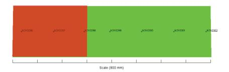
Figure 4-1: Compression molding model with Moldflow, green: final cavity; red: initial charge position; black points: sensor positions
