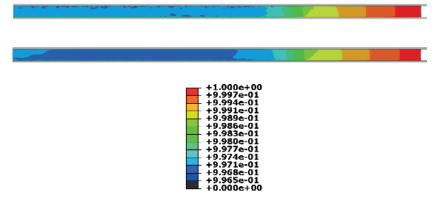
Figure 4-20: Comparison of the compressibility (det(F), see eq. 60) of the carbon UPPH SMC (top) and VE SMC (bottom) after 0.025 s simulation time
