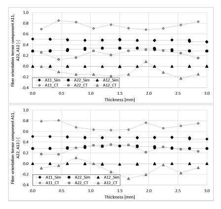
Figure 4-4: Comparison between the fiber orientation distribution from the simulation and CT-scans (from [Bry14]): CT-Position 1 at x = 339 mm, y = 200 mm (top) and CT-Position 2 at x = 431 mm, y = 200 mm (bottom)
