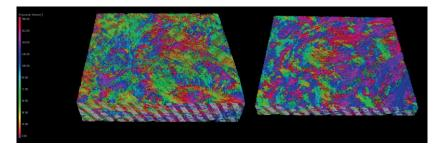
Figure 3-20: Micro tomography scan with color-coding of the fiber orientation direction of the flow front (sample 1): view on top of the sample (left) and sliced in the middle (right).
