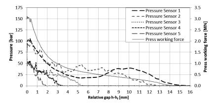
Figure 3-7 Emplary pressure distribution of the UPPH carbon fiber SMC for a closing speed of  $\dot{h} = 1 \text{ mm s}^{-1}$  [Hoh17b]
