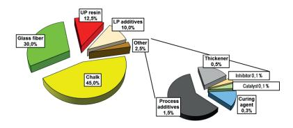
Figure 2-1: Composition of a typical Class-A SMC in wt.-% [Hoh15]
