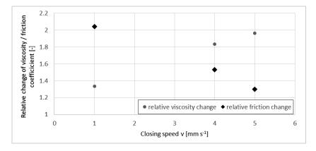
Figure 3-16: Relative change of the extensional viscosity and hydrodynamic friction between the initial charge area and the flow area of the UPPH carbon fiber SMC [Hoh17b]
