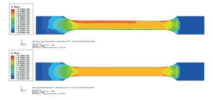
Figure 5-13: Von Mises stresses of the deformed tensile bars: mapped fiber orientation (top) and quasi-isotropic fiber orientation (bottom) from the IRTG reference structure
