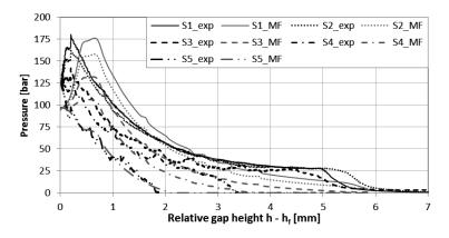
Figure 4-2: Comparison between the pressure distribution from the experiments (black) and the commercial simulation tool based on the fitted reactive viscosity model (grey)
