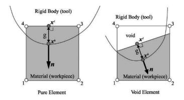
Figure 2-13: Definition of the penetration for pure and void elements [Ben04]
