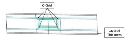
Figure 4-25: Blocking of the Eulerian mesh of the IRTG reference structure
