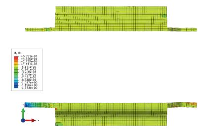
Figure 4-27: Displacement of the tapes during the compression molding process in flow direction
