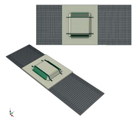
Figure 4-24: Initial configuration of the process simulation of the IRTG reference structure with the local unidirectional reinforcements (green) and the initial charge (beige)
