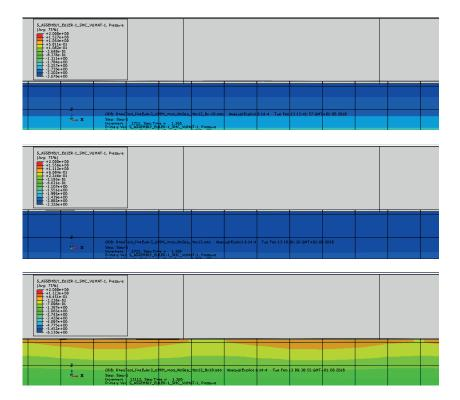
Figure 4-11: Evaluation of the penetration of the SMC through the mold surface depending on the bulk viscosity parameter: reduced (top), original (middle) and increased parameter set (bottom)
