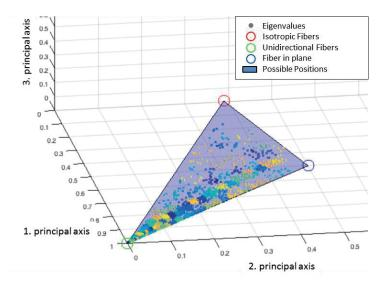
Figure 5-7: Clustering of material properties based on the eigenvalues of the fiber orientation tensor. Nodes in the same clusters have the same color. [Mey16]
