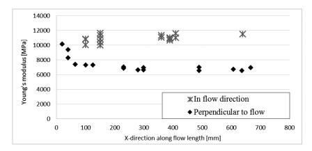
Figure 4-6: Progression of the Young's modulus over the plate length in and perpendicular to the flow direction (data from Mrkonjic et al. [Mrk15])
