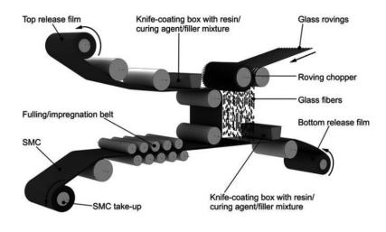
Figure 2-2: Principle of SMC production [Che16]
