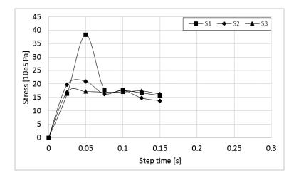
Figure 4-19: Simulated stress distribution for Sensor 1 to 3 for the carbon UPPH-SMC material
