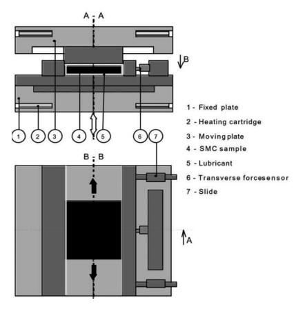
Figure 2-7: Schematic illustration of the plane strain/channel flow rheometer. To gain plane strain, a 1D flow is enforced [Dum03]
