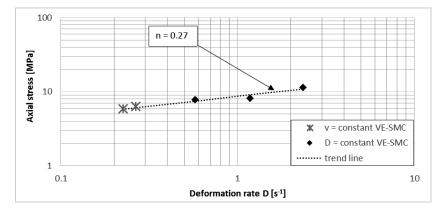
Figure 3-13: Fitting of the viscosity power-law exponent n with the results for the constant nominal deformation rates (D =  $0.5 \text{ s}^{-1}$ ,  $1.0 \text{ s}^{-1}$  and  $2.0 \text{ s}^{-1}$ ) and the constant closing speed ( $\dot{h} = 1 \text{ mm s}^{-1}$ ) of the VE-SMC formulation [Hoh17a]
