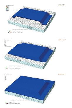
Figure 4-14: Results of a test mold filling simulation during the development process
