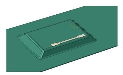
Figure 5-11: Position of the tensile bar in the IRTG reference structure
