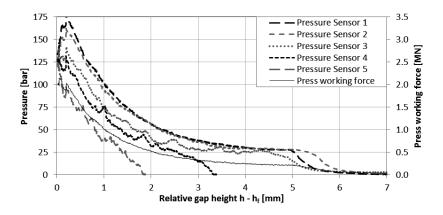
Figure 3-3: Exemplary pressure distribution of the standard Class-A SMC for a closing speed of  $h = 1 \text{ mm s}^{-1}$
