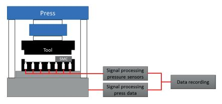
Figure 3-2: Experimental setup for the rheological measurements
