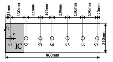
Figure 3-1: Position of the SMC initial charge and the pressure sensors along the lower mold part of the rheological tool [Hoh17a]
