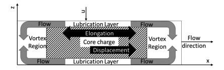
Figure 3-23: Schematically cross-Section of the probable flow of glass fiber UPPH SMC during the molding process
