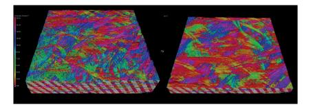
Figure 3-21: Micro tomography scan with color-coding of the fiber orientation direction of the sample from the center region (sample 2): view on top of the sample (left) and sliced in the middle (right).
