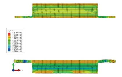
Figure 4-29: Displacement of the tapes during the compression molding process in compression direction (bottom)
