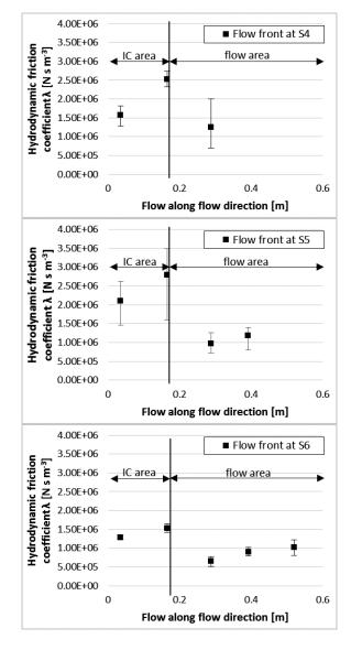
Figure 3-14: Progression of the hydrodynamic friction coefficient  $\lambda$  over time and location for the UPPH carbon fiber SMC and a constant closing speed of  $h = 1 \text{ mm s}^{-1}$ [Hoh17b]
