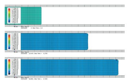
Figure 4-16: Evaluation of the flow front with the compression stresses at t = 0 s (top), t = 0.375 s (middle) and t = 0.75 s (bottom)
