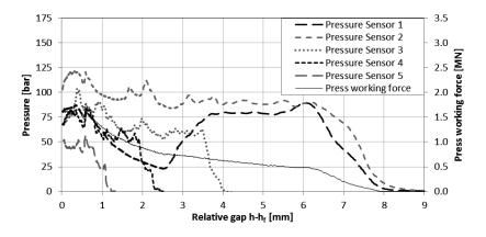
Figure 3-5: Exemplary pressure distribution of the VE-SMC for a closing speed of  $\dot{h}$  = 1 mm s^{-1}
