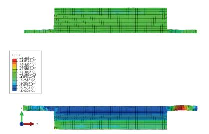
Figure 4-28: Displacement of the tapes during the compression molding process in-plane perpendicular to the flow direction
