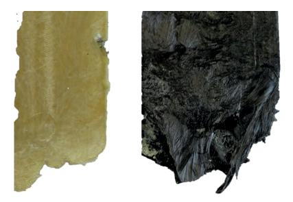
Figure 3-17: Comparison of the fiber bundle structure in the glass fiber reinforced VE SMC (left) and the UPPH carbon fiber SMC (right)
