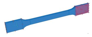
Figure 5-12: Boundary conditions and loads of the tensile bar specimen
