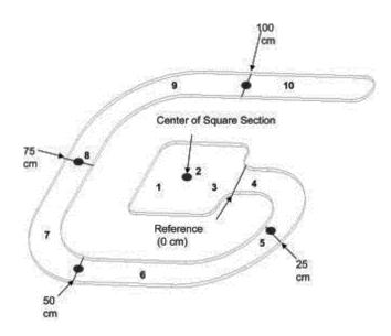
Figure 2-8: Schematic illustration of a spiral flow tool [Rab08]
