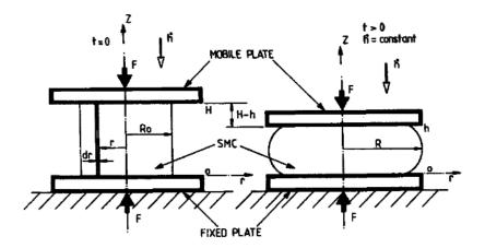
Figure 2-5: Schematic illustration of the squeeze flow rheometer [Sil81]
