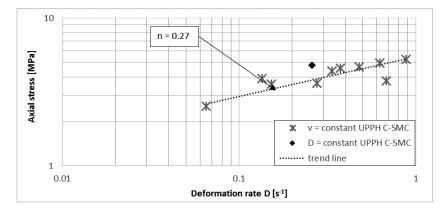
Figure 3-15: Fitting of the viscosity power-law exponent n with the results for the constant nominal deformation rates (D = 0.25 s<sup>-1</sup>) and the constant closing speed ( $\dot{h}$  = 1 mm s<sup>-1</sup>) of the UPPH C-SMC formulation
