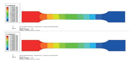
Figure 5-14: Displacement of the deformed tensile bars: mapped fiber orientation (top) and quasi-isotropic fiber orientation (bottom) from the IRTG reference structure
