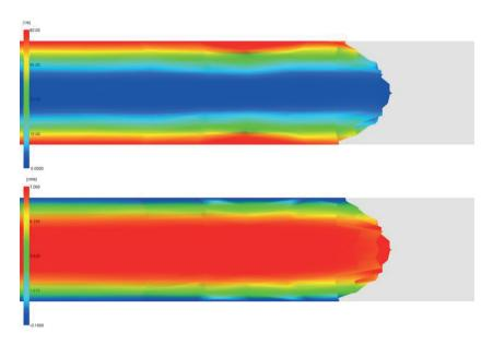
Figure 4-5: Shear rate (top) and velocity in flow direction (bottom) at the flow front during the compression molding simulation with the commercial simulation tool
