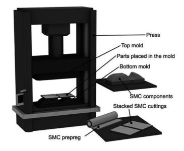
Figure 2-3: Process steps for the manufacture of SMC components with cutting, stacking, placing of the initial charge in the mold and the final part [Che16]
