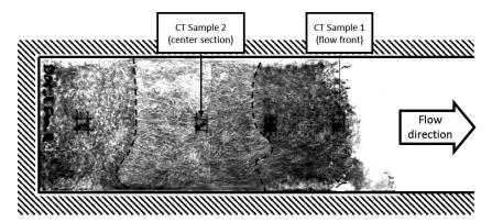
Figure 3-18: Gray-scale picture with high contrast of a UPPH glass fiber SMC short shot and CT Sample positions
