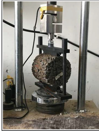
Fig. 2. The process of splitting strength test.
