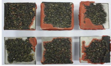
Fig. 3. Failure modes of adhesive strength test
