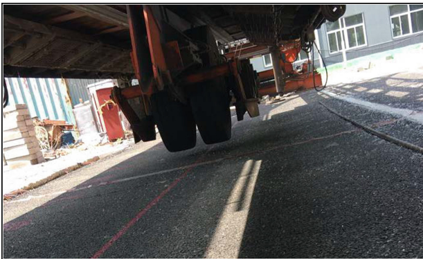
Fig. 3. The test road and accelerated loading equipment.
