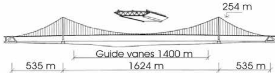
Figure 2.17 Great Belt Bridge (from [p])
