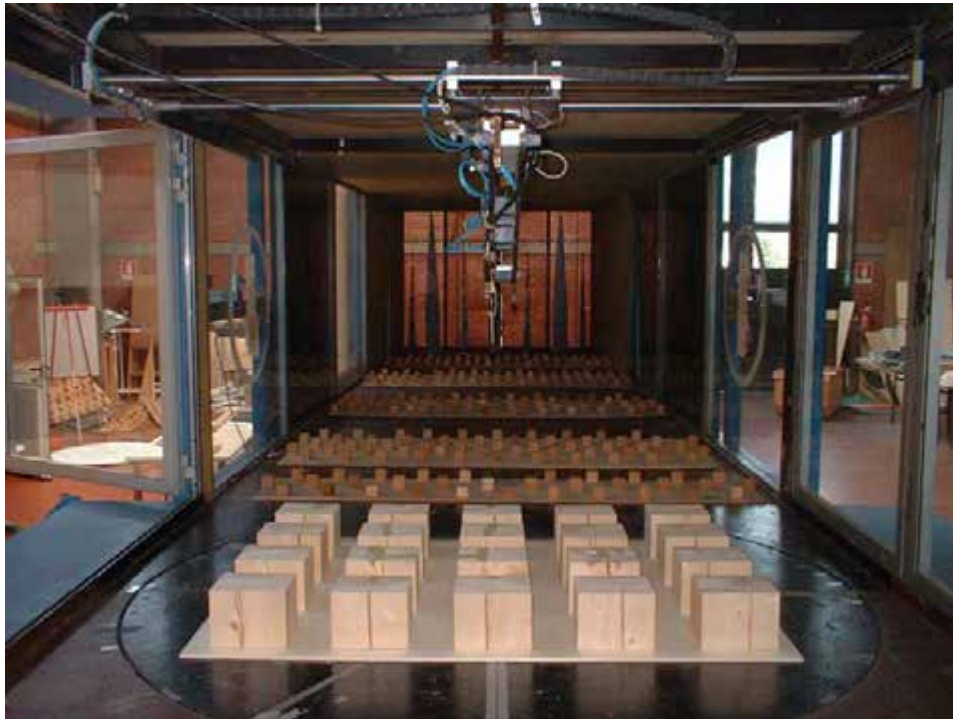
Figure 5.6 Model of urban area in the CRIACIV wind tunnel
