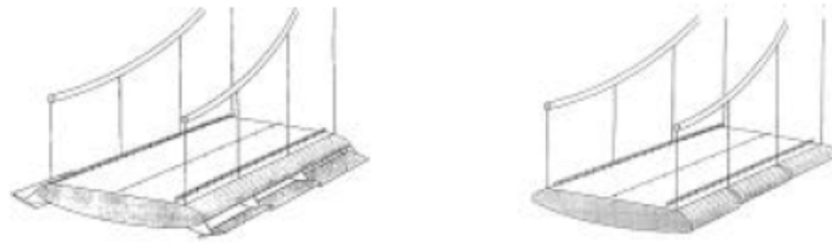
Figure 2.29 Sections with flaps on pylons and integrated in the section (from am])
