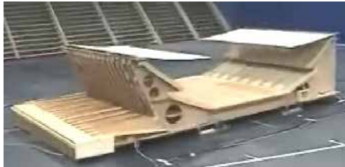
Figure 4.1 Aeroelastic model tested in the Politecnico di Milano boundary layer wind tunnel.
