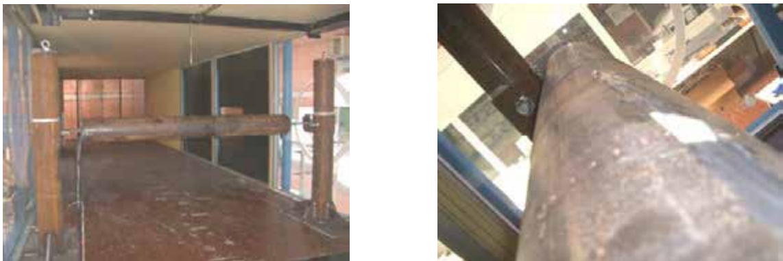
Figure 4.9 The cable model tested in the BLWT of CRIACIV in Prato.
