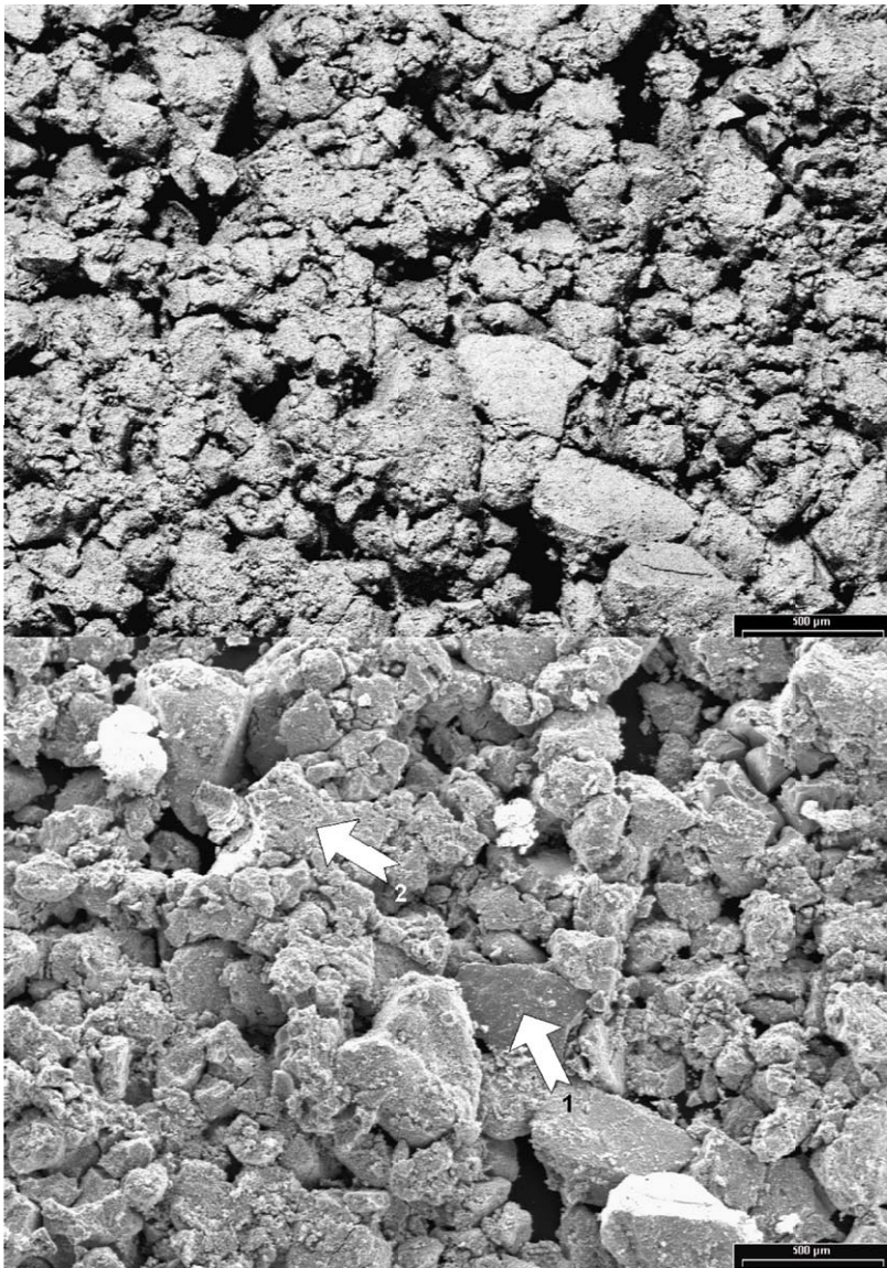
Figure 99: Microphotograph taken with SEM of the ashes of microbial biomass loaded with the removed metal obtained from the muffle kiln. Top: microphotographs taken by utilising the re-emission or reflection of high energy electron belonging to the primary ray, useful to the identification of the substances present. Bottom: microphotograph of the same area, taken by utilising the emission of secondary low energy electrons, technique used to take pictures with a resolution up to 5 nm. In this picture the two points in which the dot-like analysis were carried out are indicated. The points were chosen as they responded in a different way to the primary electrons, as it is possible to see from the different colour shown in the top photograph.
