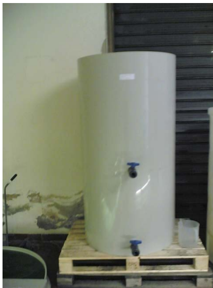
Figure 51: Decanter used to concentrate biomass. The valve at the top was used to let the medium flow away, while the valve at the bottom was used to collect the concentrated biomass.
