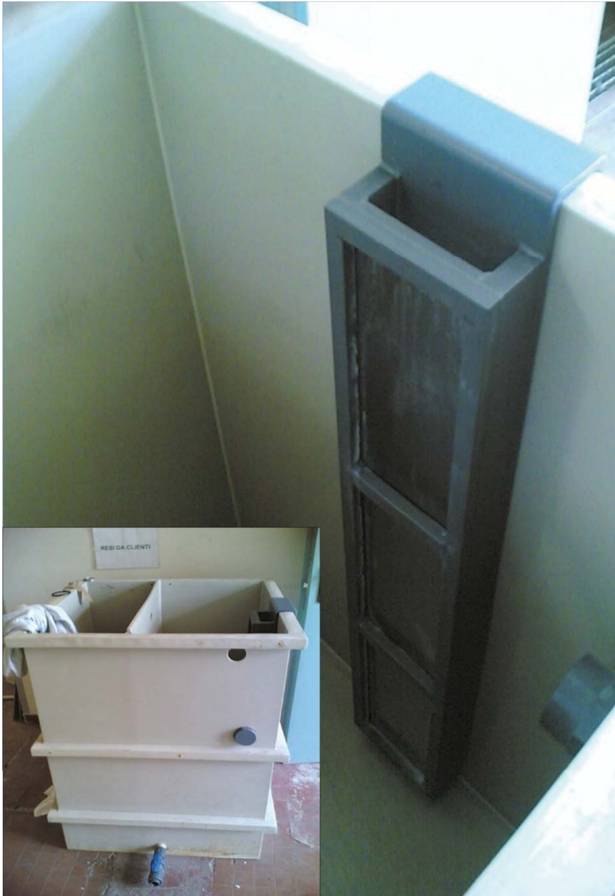
Figure 62: Dialysis cell inside the tank used for the experiments. Detail: Experimental tank with the dialysis cell hung at its right edge.
