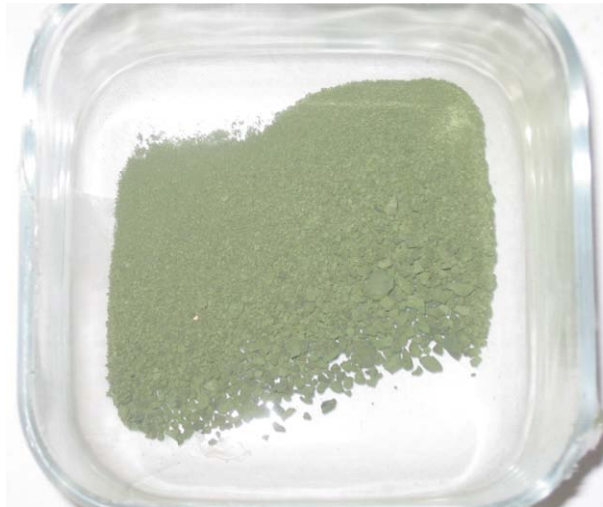
Figure 96 : Ashes obtained after the treatment of the microbial biomass in muffle kiln.
