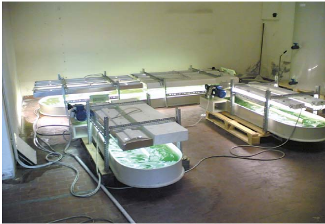
Figure 50: Raceway pond of 250 L and 500L volume used for Nostoc PCC7936 culture, illuminated by fluorescent lamps positioned above the ponds.
