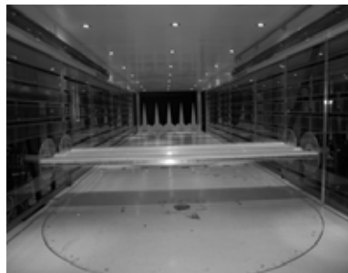
Figure 3: Sectional model of the deck in the wind tunnel working section: a) during tests of the windward deck, b) during tests of the leeward deck;
