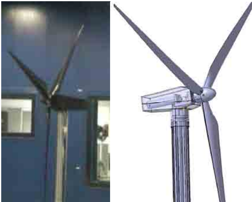
Figure 1: 1:50 scaled model of the wind turbine (left) and 3D rendering of the model (right)
