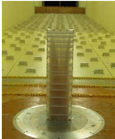
Figure 1: Pressure-tapped benchmark building model inside wind tunnel.
