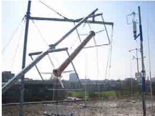
Figure 31: Rain-Wind induced vibrations experimental device
