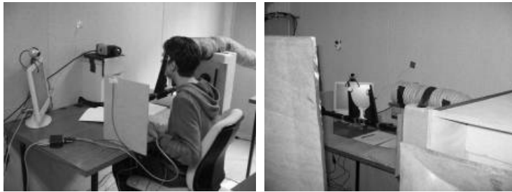
Figure 2: Experimental zone with an air duct on the right side of the subject, an infrared camera in front of the subject and a head position system in order to ensure a good impact area.
