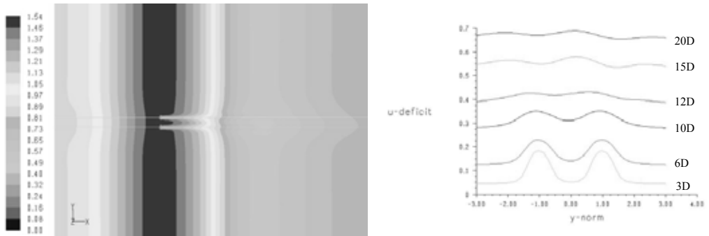
Figure 2: normalized x-velocity contours and velocity deficit – realizable k-ε
