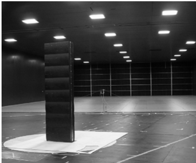
Figure 1: Building wind tunnel model. The elastic suspension system is under the false floor and allows for model oscillations
