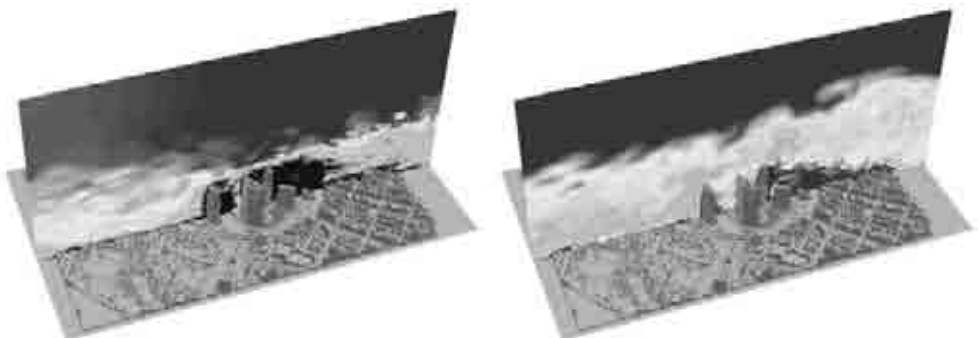
Figure 2: Instantaneous streamwise velocity and temperature field in the roughness layers over the actual city.
