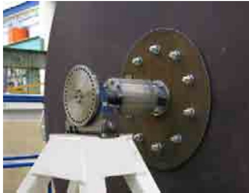
Figure 2 Turntable and force transducer configuration
