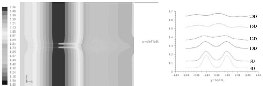
Figure 3: normalized x-velocity contours and velocity deficit – RNG k-ε
