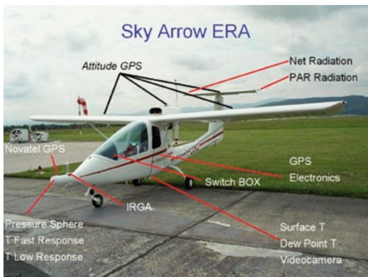
Figura 5. Sky Arrow ERA (Environmental Research Aircraft)
