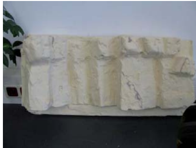
Figure 7: Detail of the passion, death and resurrection of Jesus Christ, CNC milled in model material
