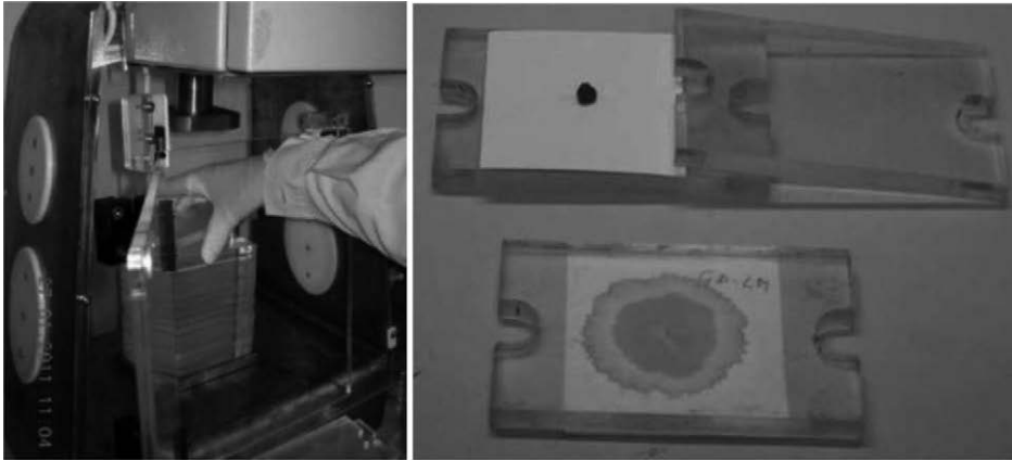
Figure 23 - Hydraulic press (left) and plexiglass plates before and after compression (right)
