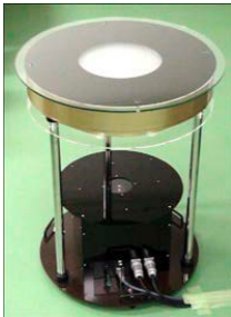
Fig. 6. Portable 360-degree viewable 3D display, “Holo-Table”.
