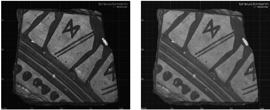
Figure 2: Texture images of fragment G741, left: fringe projection, right: SfM
