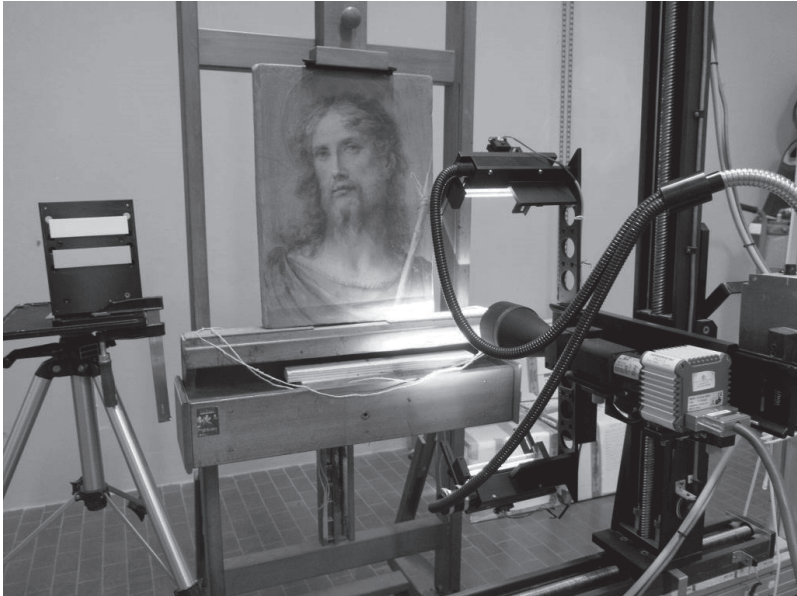
Fig. 1 Vis and NIR hyper-spectral imaging scanner developed at IFAC-CNR
