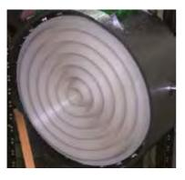
Fig. 1: Dummy load for HPM  $TM_{011}$  calorimeter.
