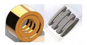
**Fig. 1:** a) The antenna mesh plot in vertical plane, b) Finite element simulation of our antenna in vertical plane V/m.
