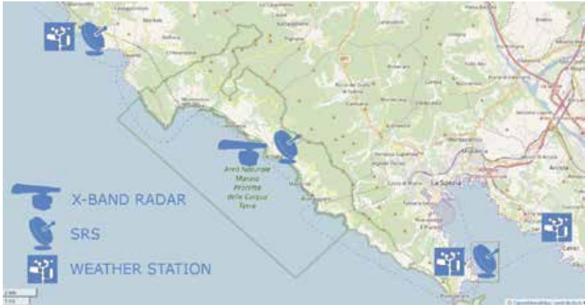
Figure 1 – Environmental monitoring sensors installed at the east Liguria field test sites.
