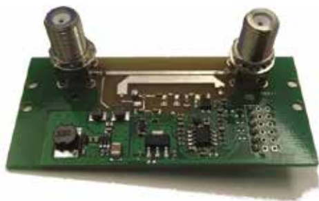
Figure 4 – SRS sensing board: the two F connectors provide connectivity towards the satellite television decoder (left) and to the LNB (right).
