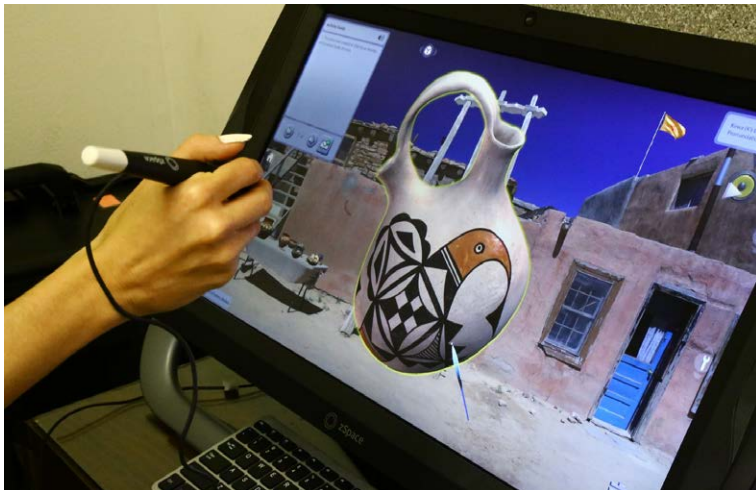
Figure 3. A user interacting with an object in the zSpace ® 200 mixed reality environment.
