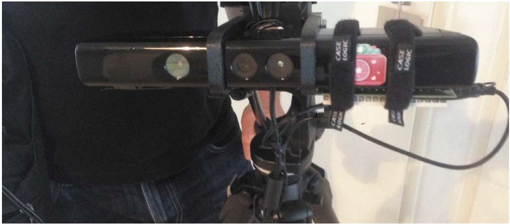
Fig 1. Kinect based DIY portable volumetric capture system 2018, Daniel Buzzo, sensor head and control hardware, Copyright the author.
