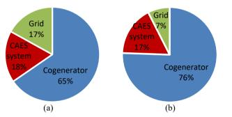
Figure 8 - Coverage of electricity needs for the 1560 kW scenario (a) and the 2000 kW scenario (b).
