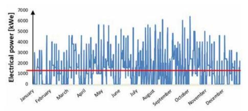
Figure 7 - Annual trend of electrical energy required by ships at berth. The red line indicates the average over the year analysed.
