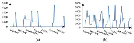
Figure 3 - Trend of electrical energy demand (kWh) of ships at berth during January (a), July (b).
