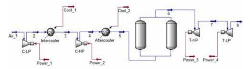
Figure 6 - Plant layout of a CAES system.
