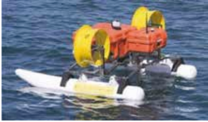
Figura 2 - DEVSS, autonomous surface vehicle . Figure 2 - DEVSS, autonomous surface vehicle .
