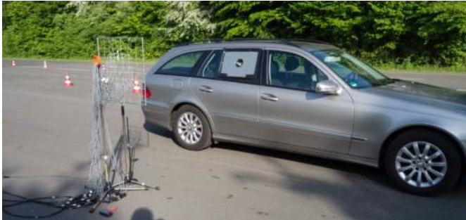
Figure 4.10.: Setup of the pass-by measurement. The spiral microphone array and the photoelectric sensor were set 1.5 meter from the near-side surface of the car.
