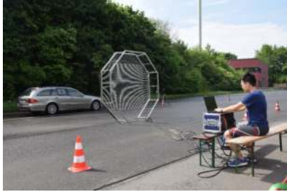
(a) Car01 pass-by measurement.
