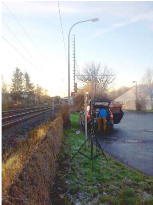
Figure B.3.: The setup of the train pass-by measurements.
