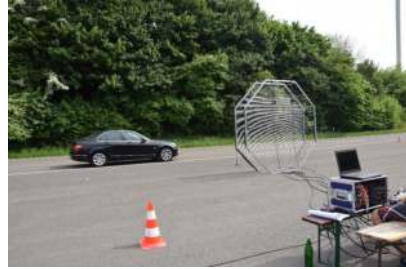
(b) Car02 pass-by measurement.
