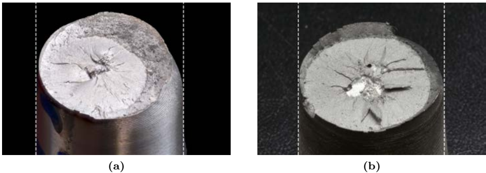
Figure 3.14: a) Necking for 1.6220 specimen U20O2 at \Delta\sigma = 280 MPa; b) No pronounced necking for 1.6760 specimen U22M6 at \Delta\sigma = 280 MPa
