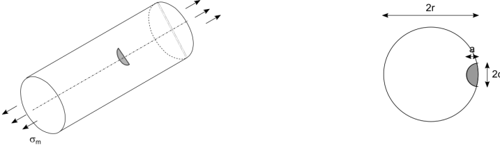
Figure B.3: Cylinder with semi-circular surface crack [161]
