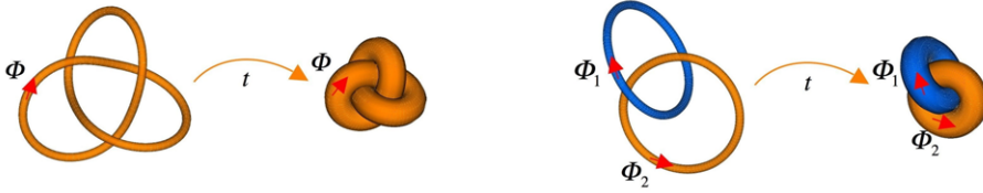
Fig. 13.1: Ideal relaxation of a magnetic trefoil knot and a Hopf link.
