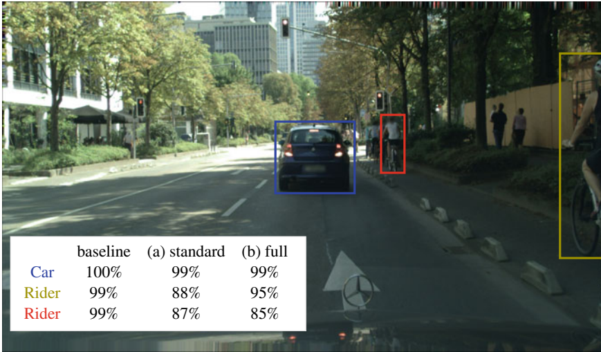
Fig. 2 Qualitative example of position-dependent confidence calibration on a Cityscapes image with detections obtained by a Mask-RCNN. First, standard calibration is performed using similar confidence estimates \hat{p} without any position information. This results in rescaled but still similar calibrated confidence estimates (note that we have distinct calibration models for each class). Second, we can observe the effect of position-dependent calibration using the full position information (position and shape) as the two riders with similar confidence are rescaled differently. When using all available information, we can observe a significant difference in calibration since both, position and shape, have an effect to the calibration
