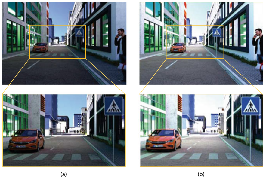
Fig. 3 Left a : Synthetic images without lens artifacts. Right b : Applied sensor lens artifacts, including exposure control
