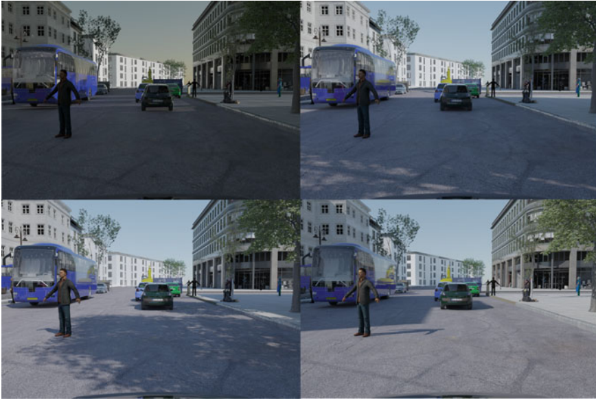
Fig. 3 Example of scene parameter variation; in this case the time of the day is varied, causing dramatic changes in the scene illumination according to contrast variations
