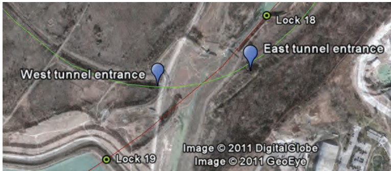
Fig. 2.8. Google Earth is used with a 1934 photo overlay to determine the exact position of the east entrance of the Grant Trunk Railroad tunnel under the third canal. (Created in Google Earth Pro, 2011.)
