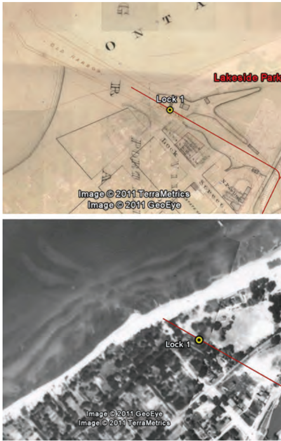
Fig. 2.6. Top: Welland Canal 1855 survey map, showing the location of the piers and Lock 1 of the first canal, overlaid in Google Earth shown faintly underneath. (Digital image: Brock University Archives, St. Lawrence Seaway Authority [Canada] Fonds, Second Welland Canal Survey Map 1, ca. 1855; reproduced in Google Earth Pro, 2011.) Bottom: 1934 air photo showing the submerged shadows of the piers. (Digital image reproduction: Brock University Map Library; NAPL photo A4700 #33.)
