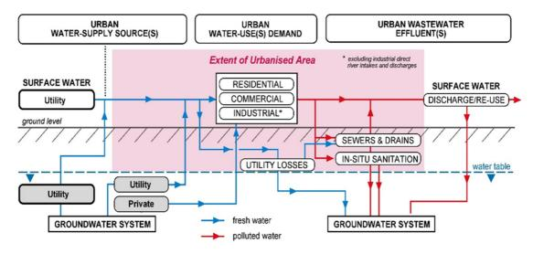
**Figure A1** Typical scheme of interaction between water utility operations and a groundwater system (after Foster 2020a).
