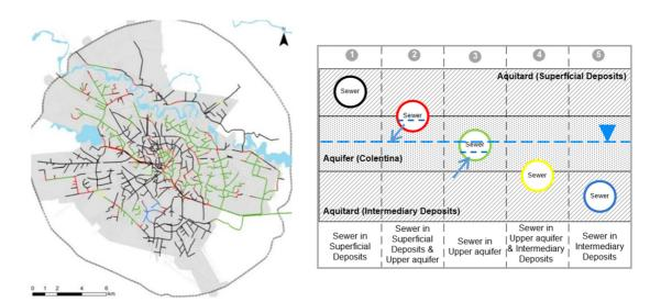
**Figure C7** Urban infrastructure data used for construction of a groundwater numerical model of the shallow aquifer system.
