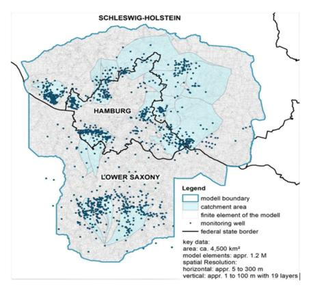
Figure C6 Configuration of Hamburg groundwater numerical model.
