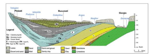
Figure C8 Hydrogeological cross-section of the Bucharest area.
