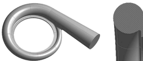
Figure 1. Geometrical shape of the investigated volutes.
