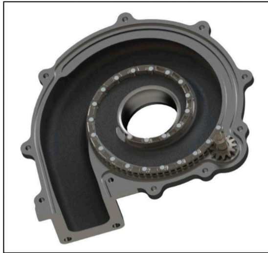
Figure 11. Rear housing w links, rollers, and gear.
