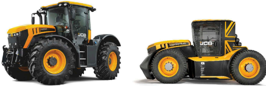
Figure 7. Production Fastrac bonnet (L) was carried-over to the WFT (R), restricting the opportunity to create space for two-stage turbocharging.
