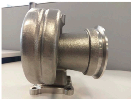
Figure 9. Sample thin-wall turbine housing without insulation.
