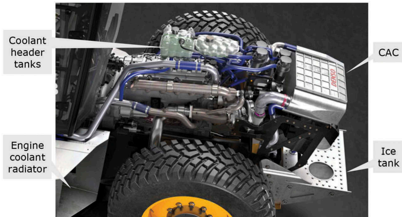
Figure 13. Charge air cooling and ice tank installation.
