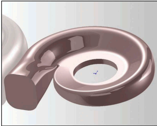
Figure 9. Volute core at full open.
