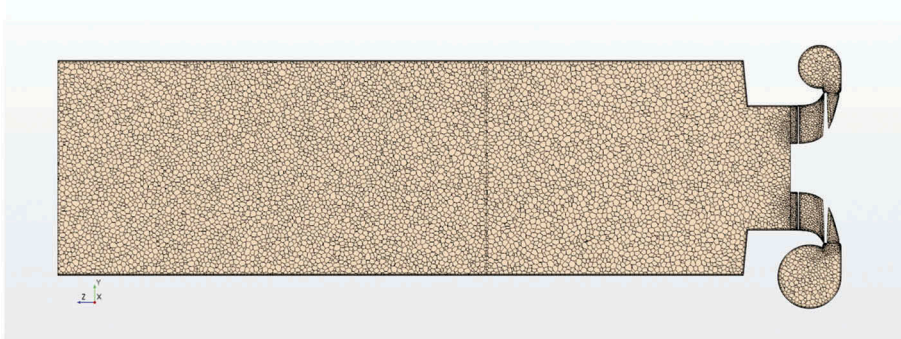
Figure 10. Section plane view of the mesh: normal to x (inlet pipe direction).
