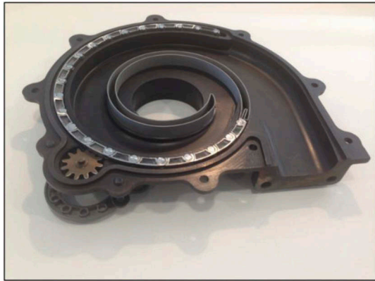
Figure 39. Special insert as exemplar to assess the leakage flow around the links.
