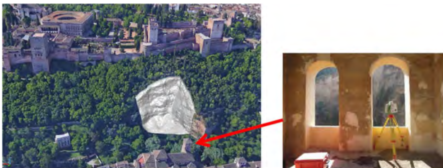
Figure 4. TLS monitoring from the bell tower of San Pedro church.
