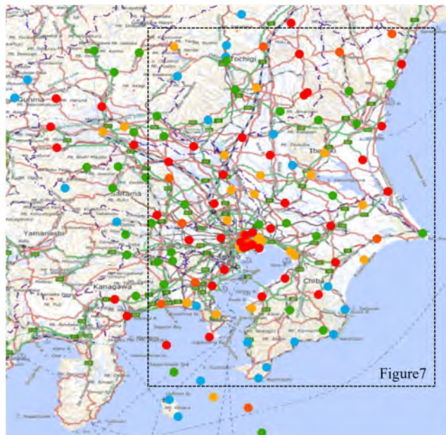
Figure 6. Judgment result in the Kanto region by deep-learning of the liquefaction degree (DDL) of the Kanto region during the 2011 earthquake off the Pacific Coast of Tohoku.
