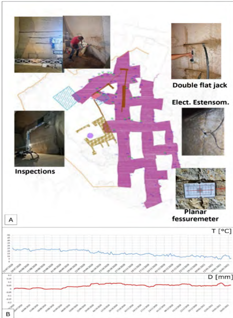
Figure 8. Set up of the monitoring system: a) plan view; b) temperature and movement data during the monitoring period.
