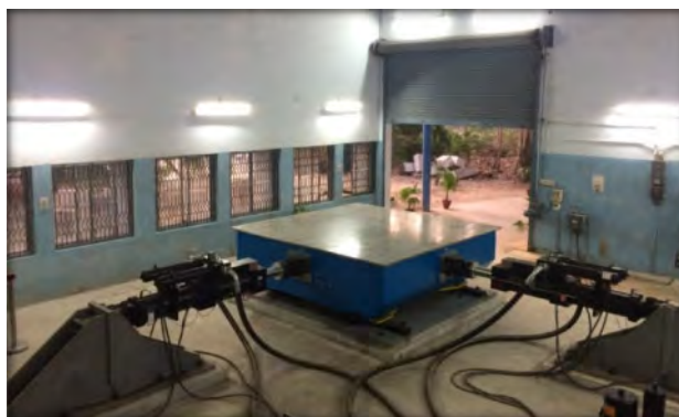
Figure 7. Biaxial 3.0x3.0m shake table test facility at structural dynamics laboratory at IIT Madras.
