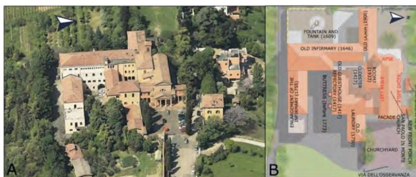
Figure 1. (A) Aerial view of the Osservanza church and of the adjacent Convent in their present configuration. (B) Plan view with indication of the main parts of the religious complex.
