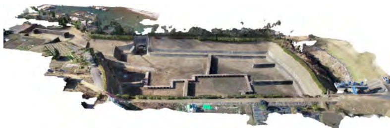
Figure 9. Perspective view of the 3-D texture model viewed from southeast direction. The size of the lumberyard, the length 100 m, the width 50 m, and depth is about 10 m.
