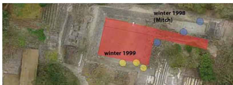
Figure 20. Aerial photo of the Copan Acropolis (east at top) showing approximate positions of tunnel collapses after hurricane Mitch (1998 in blue, and 1999 in yellow), with the position of the East Court membrane marked in red (modified after Lacombe et al., 2020).
