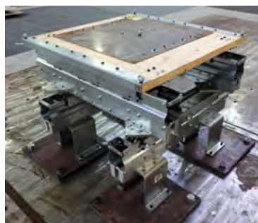
Figure 2. KSJ bidirectional isolator for seismic protection of statue-like structures.
