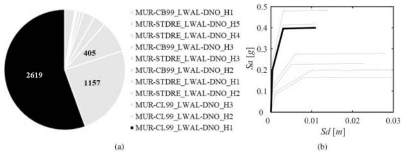
Figure 3. (a) Pie chart presenting the different masonry building classes in the Thessaloniki municipality and (b) corresponding capacity curves characterizing their nonlinear behaviour. The case-study building in class is highlighted in black.
