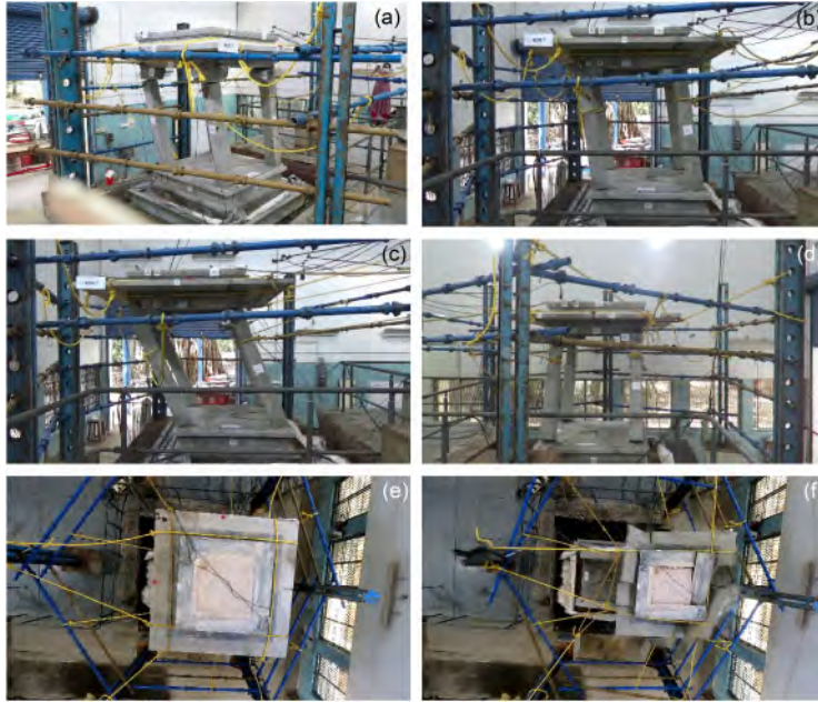
Figure 11. Images from video capture during Run-7 (a)-(b) Overturning mechanism with hinges at the bottom and top of the corbels in the lead pillars versus the rear pillars, respectively; (c)-(d) side views of the model at the verge of collapse; (e) top view of the model at initiation of mechanism; (f) top view at collapse showing disintegration of the stone slabs of the sunshades.
