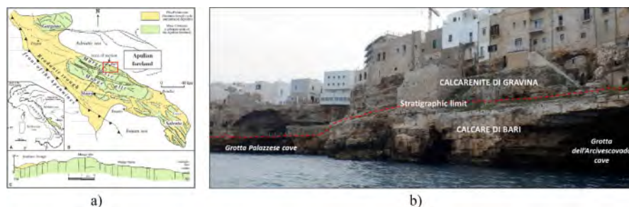
Figure 1. a) Location of the Apulian foreland in a synthetic structural map of Italy (Spalluto 2012); b) Stratigraphic limit between CB limestone and CG.
