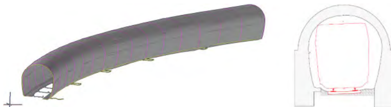
Figure 17. 3D model from geometric survey (on the left) and example of clearance overlapping (on the right): in grey the existing clearance of the tunnel, in red the clearance of the new train (PC80).
