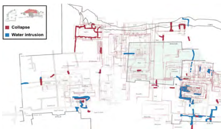
Figure 19. Map of local tunnel collapse and of water intrusion observed from 2017 to 2020 (modified after Pires, 2020).
