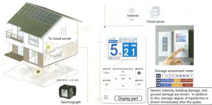
Figure 1. Damage-assessment meter for private housing development of Misawa Home Co., Ltd., Japan.
