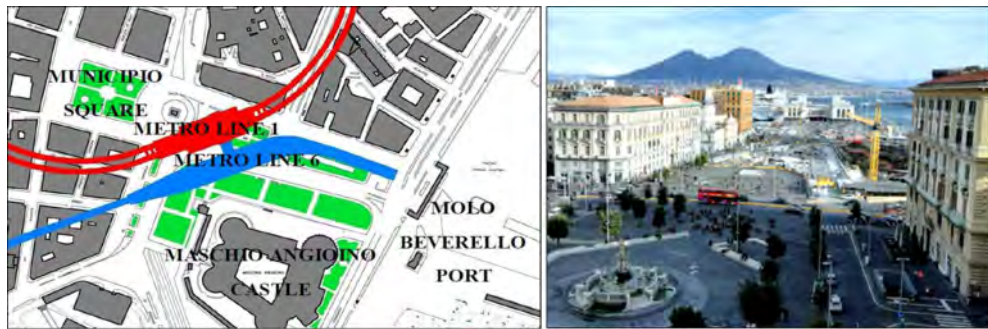
Figure 1. Municipio Station schematic plan view with highlighted (in red) Line 1 and (in blue) Line 6 and a picture of the site during construction stages.
