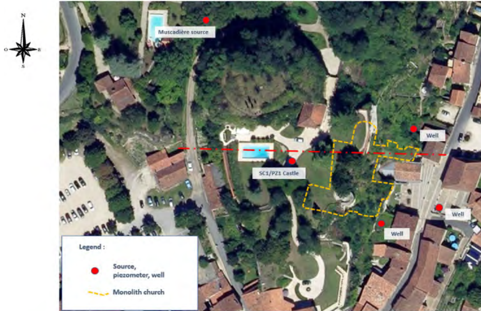
Figure 8. Position of the water level sensors on the outside and transverse cross section axis (Antea Group).
