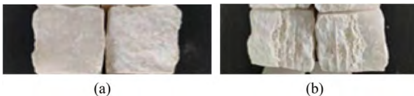
Figure 6. The failure mode of the repaired beams: (a) Group C-2, (b) Group D-3.
