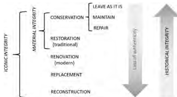
Figure 1. Conventional relationship between iconic, material and historical integrity as a function of different kinds of engineering actions.
