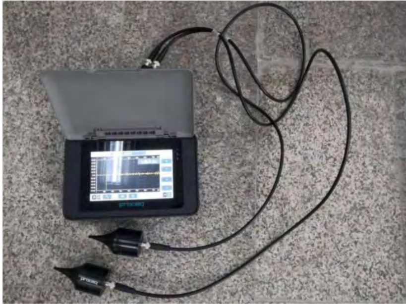
Figure 5. Type Proceq PL-200 ultrasonic apparatus.
