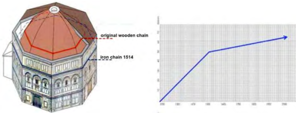
Figure 8. Left: chains position in the structure of the dome; right: outward displacement in the time.
