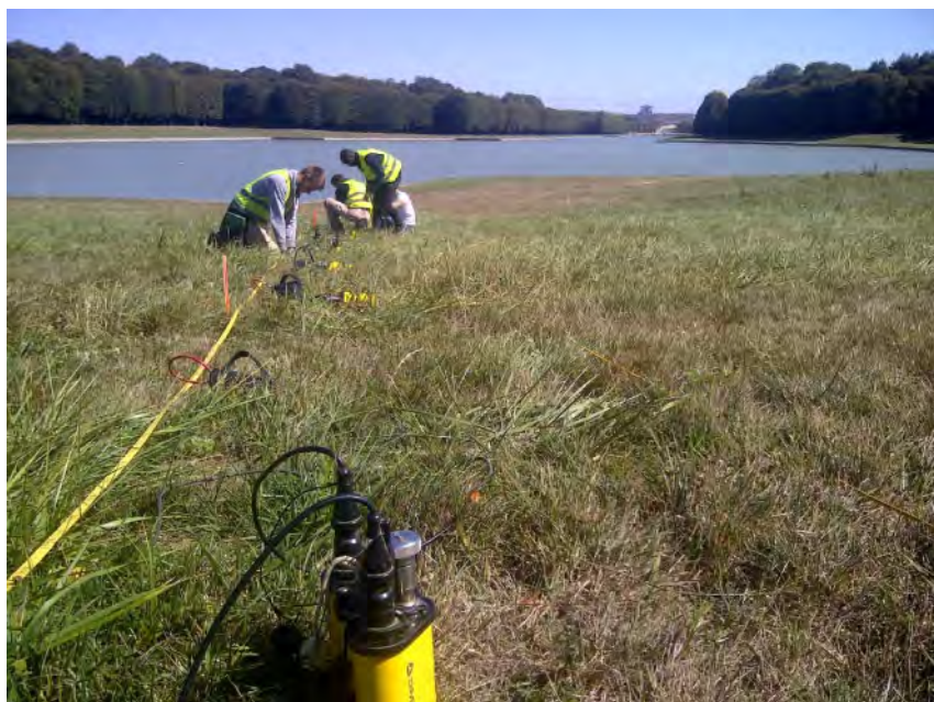
Figure 3. Installation of a base of seismic refraction measurements (Sept. 2018). The device is installed near the Gally basin. To the east, above the other end of the canal, we can see the Palace.
