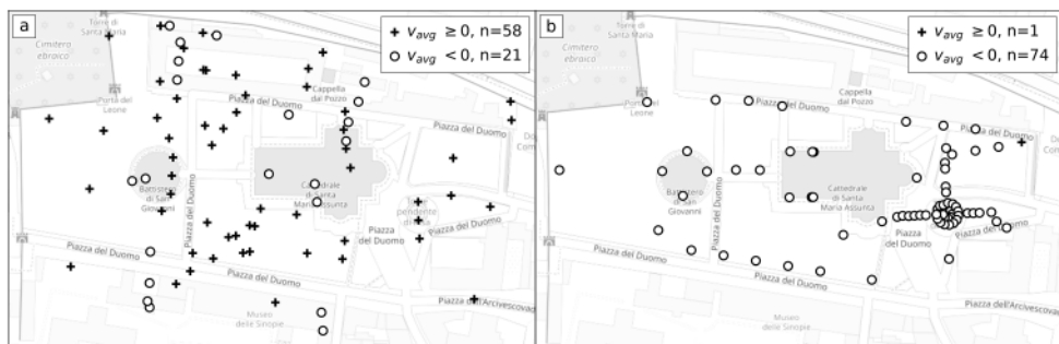
Figure 7. Sign of the average yearly settlement of Piazza del Duomo between June 2018 and 2020 as measured: (a) via Sentinel DInSAR; (b) via levelling surveys. The only cross in (b) is the deep reference point, which is considered fixed.
