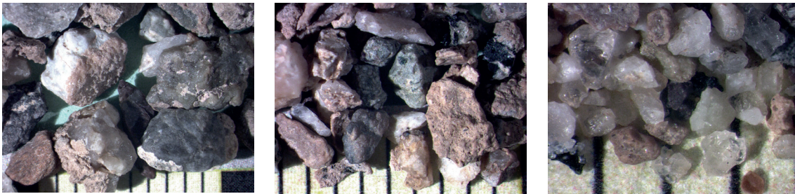
Fig. 3.18 Shapes of grains in sample 11933. Scaled in millimetre. Shape of fraction >2,000 \mu\text{m} (left), >630 \mu\text{m} (centre), >200 \mu\text{m} (right).
