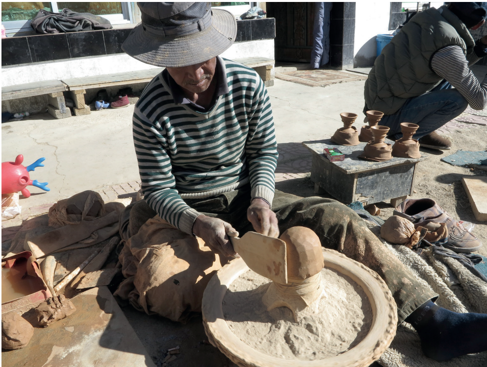
Fig. 2.6 (Top) Use of a wooden paddle to mould the clay.
