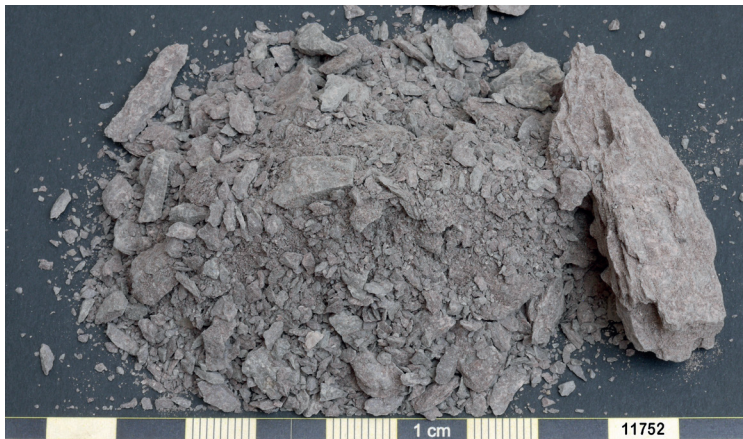
Fig. 3.41 Likir. Sample 11752. Sample colour (after Munsell): Dry 10YR 5/1 grey. Semi-dry 10YR 4/1 dark grey.
