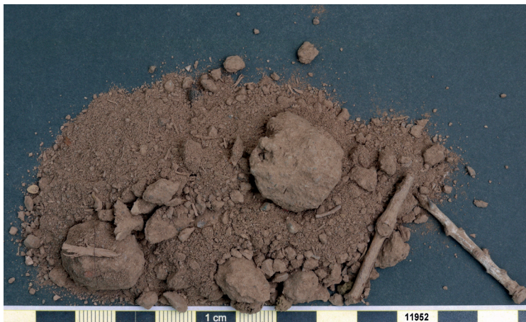
Fig. 3.26 Basgo. Sample 11952. Sample colour (after Munsell): Dry 10YR 6/2 light brownish grey. Semi-dry 10YR 3/2 very dark greyish brown.
