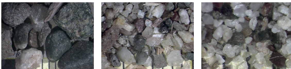
Fig. 3.27 Shapes of grains in sample 11952. Scaled in millimetre. Shape of fraction >2,000\ \mu\text{m} (left), >630\ \mu\text{m} (centre), >200\ \mu\text{m} (right).
