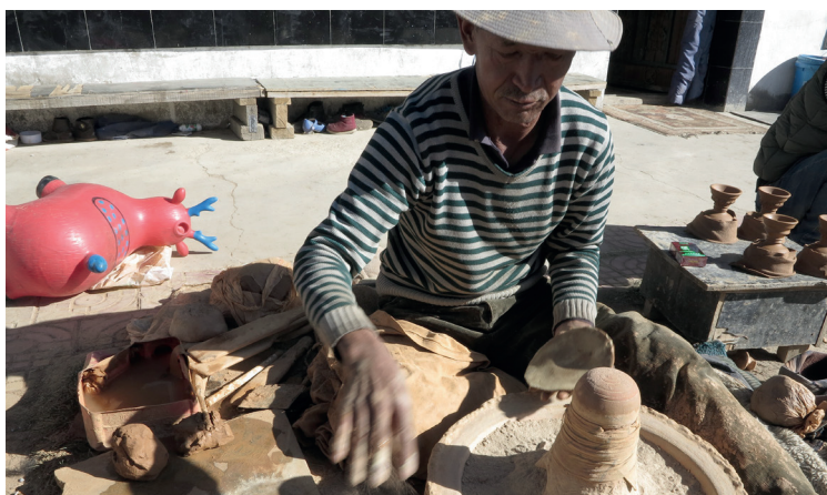
Fig. 2.5 Pottery wheel with a ceramic mould before being covered with fresh clay.
