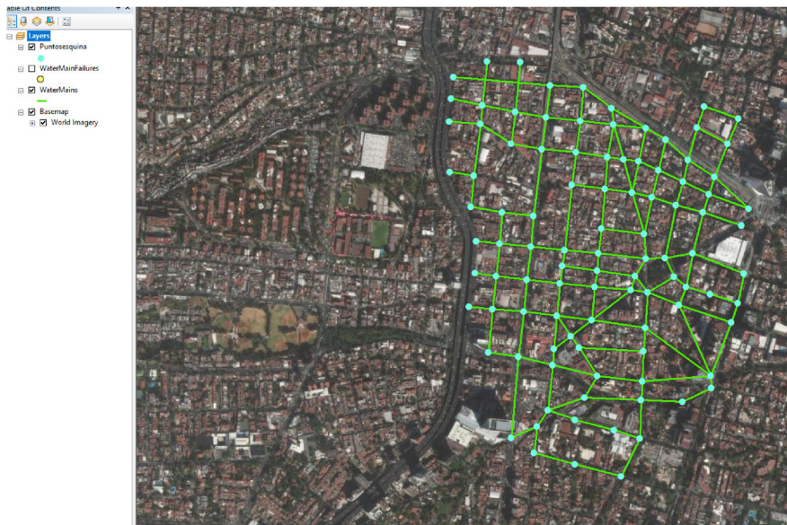
Figure 14.33 Water main grid.
