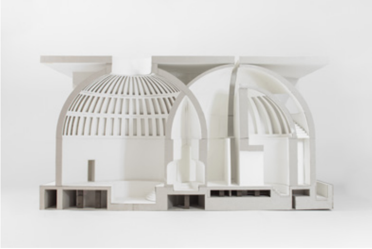
Fig. 7.3 Design for thermal baths, a model as section, scale 1:20, by Tigone Priem and Lore Delputte, students in the Studio Territory of Imagination I. Ma2 Structural Contingencies 2018–2019. Interlocking geometrical spaces, creating irregular interlocking thresholds, based on John Soane’s Bank of England.
