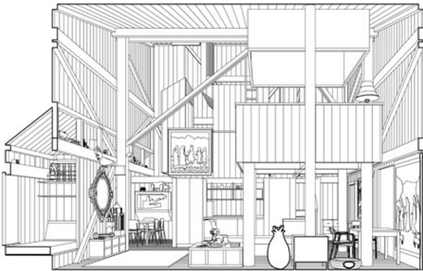
Fig. 9.3 The reimagined internal perspective of unit 9 prepared from survey drawings revealing the lived reality following on from the original propositional perspective. © Tom Coward.
