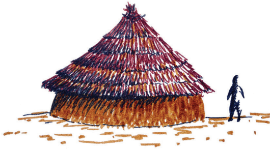
Figure 22: A Tukul near Jebel Kujur in Juba. It combines adobe for the circular wall and roofing in wood and straw
