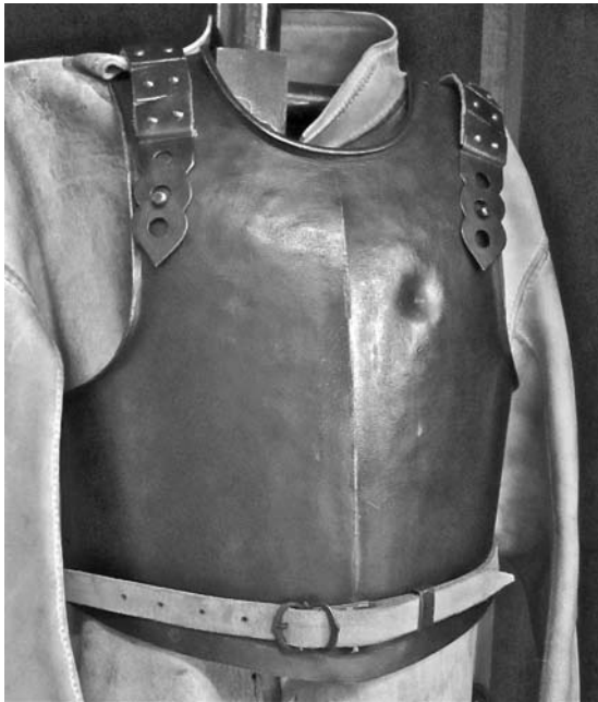
Figure 3.1 Bullet 'proof mark' on an English Civil War era breastplate (courtesy of The Stratford Armouries, Warwickshire).
