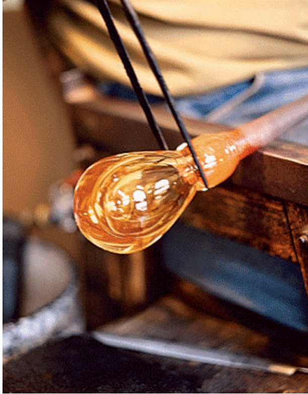
Figure 3: 'Jacking' the piece off the pipe. Photo by the author.
