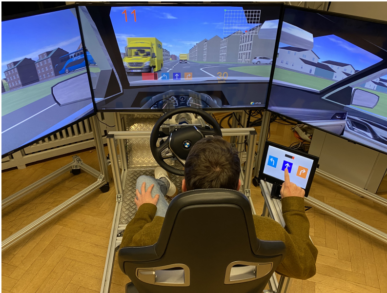
Figure 5.5: Front view of the driving simulator for highly automated driving equipped with three vehicle visualization screens (top), steering wheel and pedals (middle, unused in this experiment), a driver's seat (bottom) and a touchscreen as a maneuver decision interface (mid-right). ©2022 IEEE
