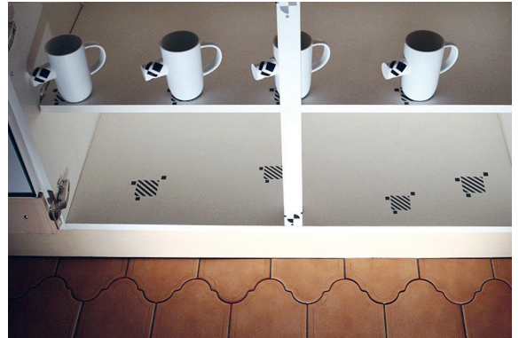
Fig. 8 Cups with handles designed for grabbing by robots and humans, stored in a cupboard deliberately without doors, and with tags marking the position of the objects. © Diego Trujillo, Source: Auger, 2014
