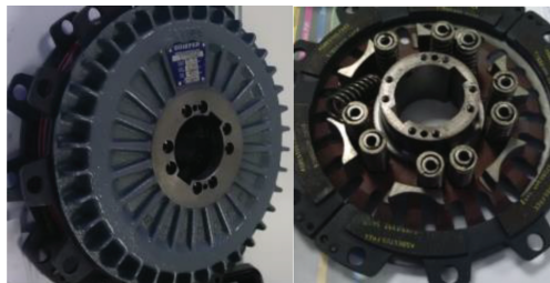
Figure 7.39 GOIZPER pneumatic Clutch Brake outside and inside.
