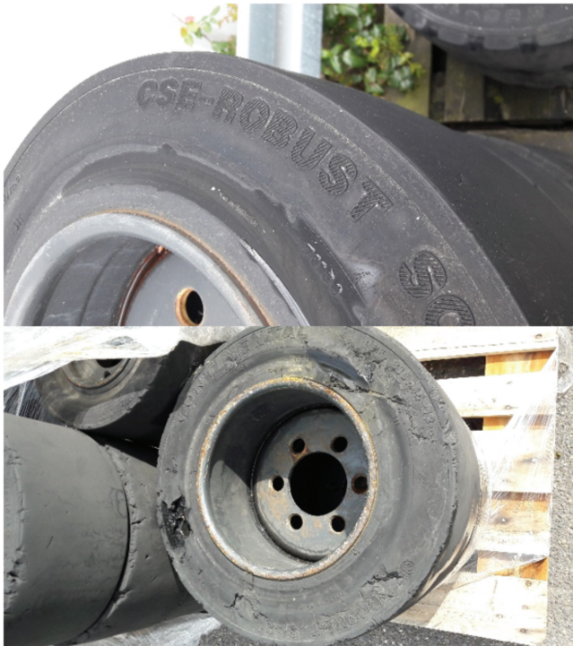
Figure 7.97 Tire changed due to wear and damage.
