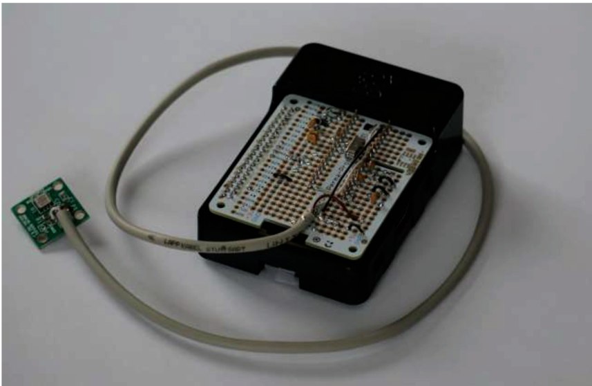
Figure 7.116 RaspberryPi based measuring system with a memS accelerometer.
