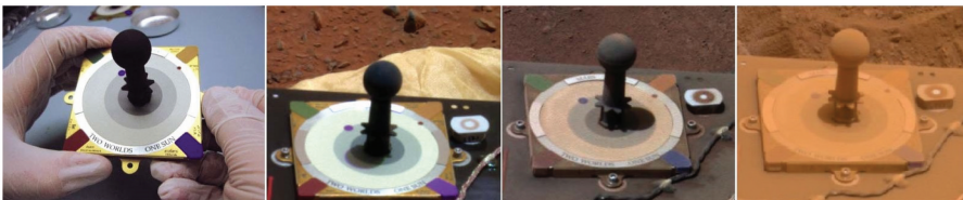
Figure 9.1 Unexpected dust accumulation on the color calibrator of a Mars rover. Without actuators for autonomous self maintenance, only the wind can help out [KinchMarsDust, 2007].
