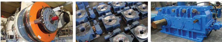
Figure 7.36 Clutch Brake (left) and gearboxes (center) by Goizper, used in Fagor's mechanical press machines (right).
