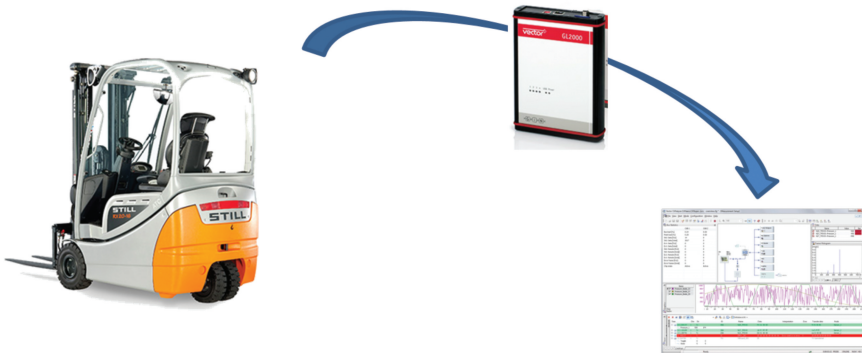
Figure 7.95 Data Logging on the internal CAN bus.
