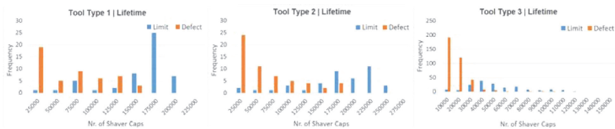
Figure 7.10 Time to failure (in amount of products) for the three main tool types.
