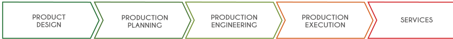
Figure 8.9 Top-down approach, where the product has all the information in every step of the value chain.
