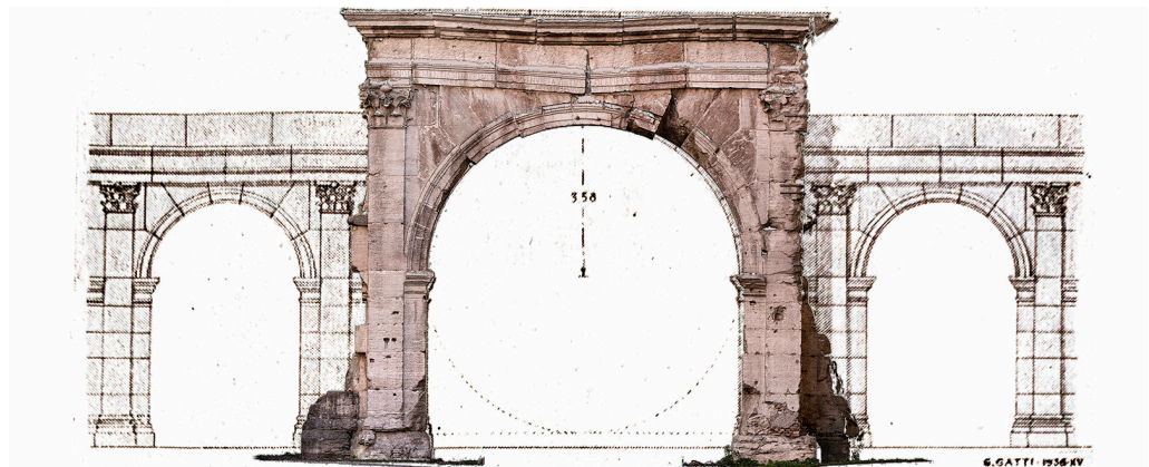
Overlapping of the photogrammetric survey with the reconstruction by Gatti [Lugli 1937].
