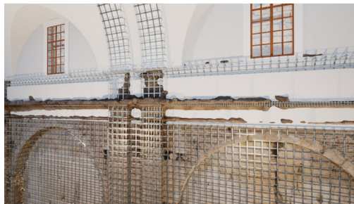
Fig. 08. Overlapping of the baroque vault on the model of the current state (graphic elaboration by the authors).
