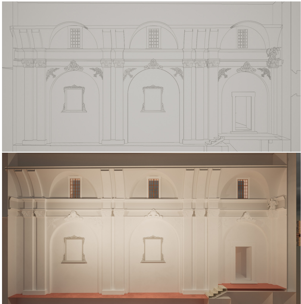
Fig. 10. Left side of the church: from the drawing of decorative apparatus to the rendering of the three-dimensional model (graphic elaboration of authors).
