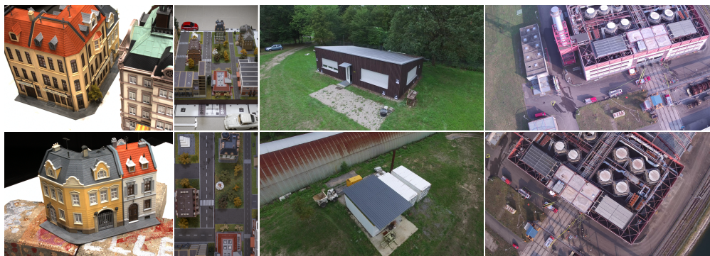
Figure 4.5: Overview of the four datasets used for performance evaluation of FaSS-MVS. Column 1: Two building models from the DTU Robot MVS dataset. Column 2: Example images in oblique and nadir view from the 3DOMcity Benchmark dataset. Column 3: Excerpt of the privately acquired TMB dataset. Column 4: Use-case-specific dataset acquired during an exercise of the local fire brigade. (Ruf et al. 2021b, Fig. 5.)
