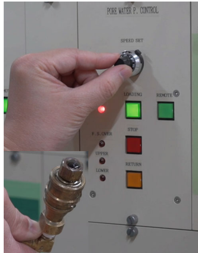
Fig. 41 Checking water coming out from the piston of servo pore water pressure
