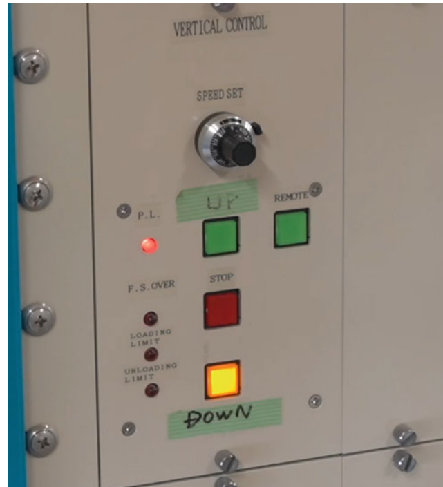
Fig. 32 Using vertical control to install vertical load cylinder
