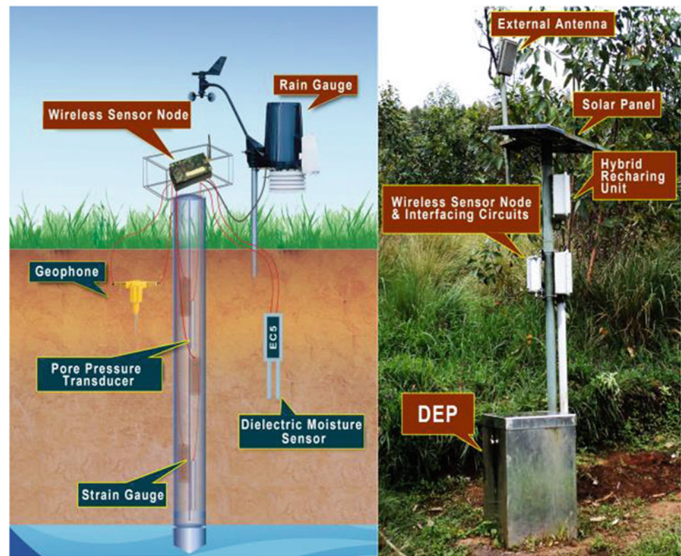
Fig. 6 Intelligent Wireless Probe with Edge Computation (Ramesh et al. 2014)
