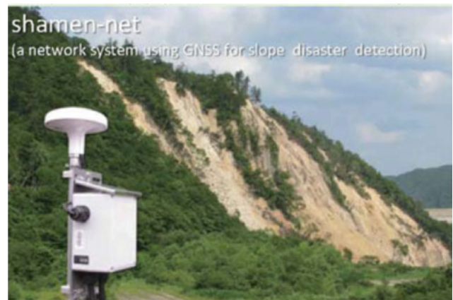
Fig. P.4 “Shamen-net” is a total monitoring system integrating GNSS and other monitoring device (Measurement precision: \pm mm, on a real time basis)
