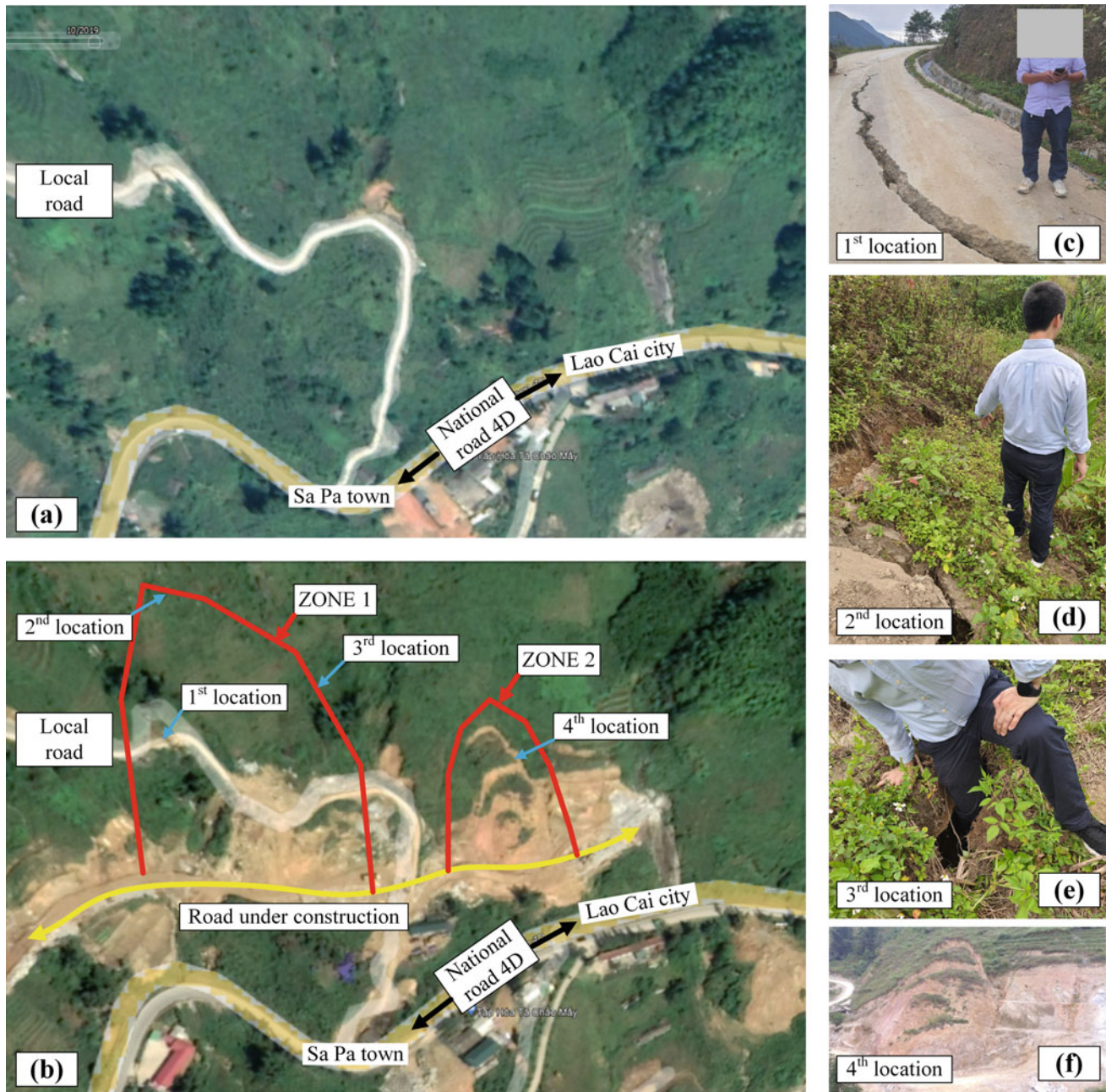
Fig. 3 Morphological changes of the slope by time and landslide views: a before road construction on October 30th, 2019; b during road construction on October 27th, 2020; c crack on local road 155; d crack
