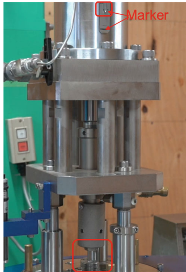
Fig. 45 Disconnecting the central axis and loading plate
