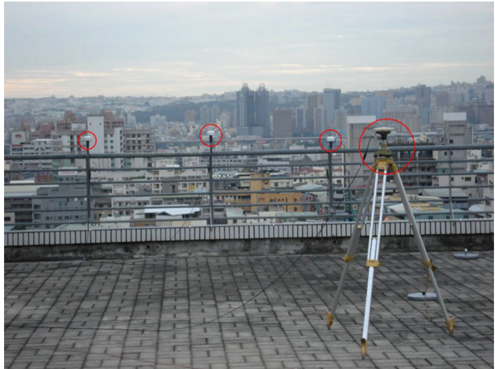
Fig. 5 Multi-antenna GPS test configuration diagram (4 mobile stations)
