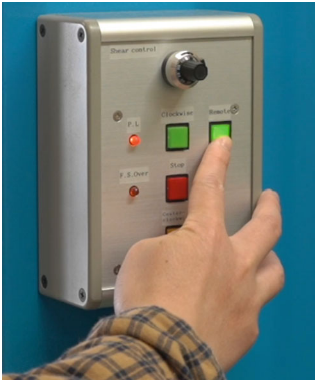
Fig. 34 Pushing the “Remote” button in the Shear control box
