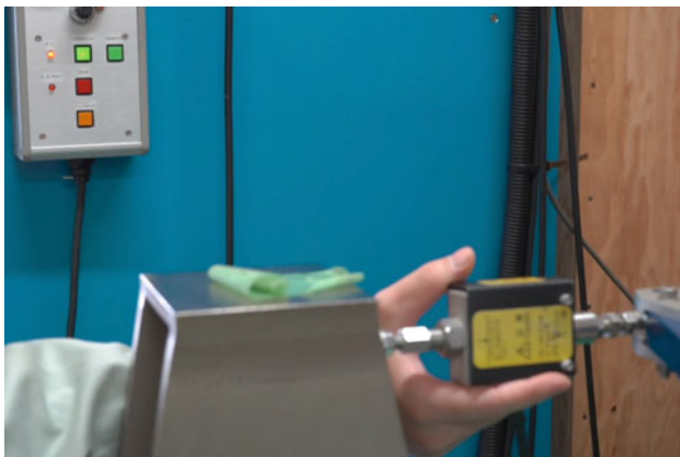
Fig. 31 Adjust the position of loading plate to install shear load cells
