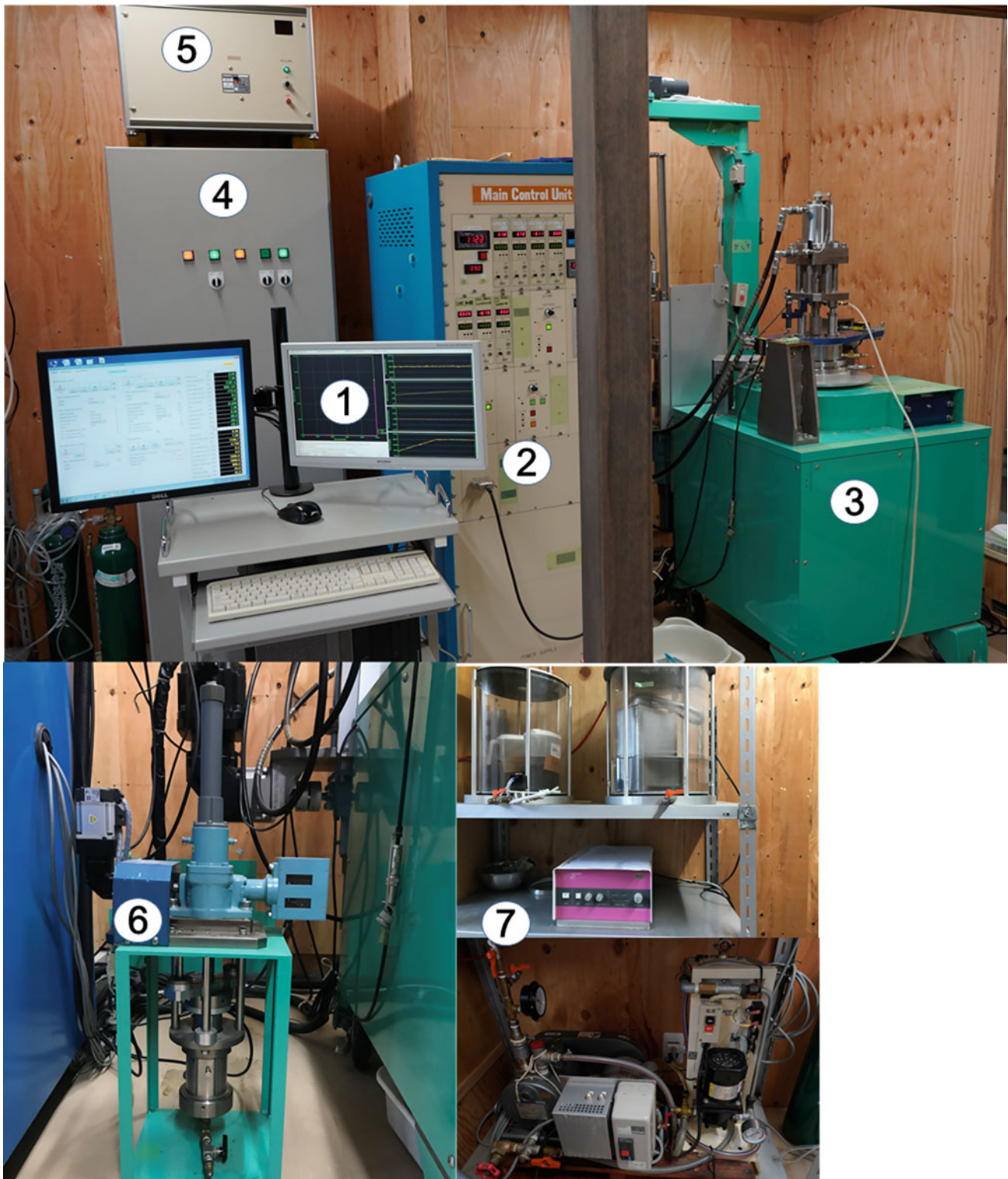
Fig. 4 Main units of the ICL-2 apparatus
