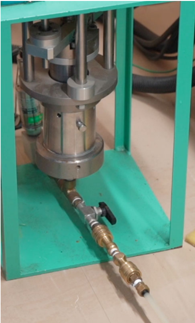
Fig. 40 Connecting the water pipe to the servo pore water pressure
