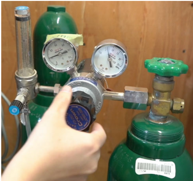
Fig. 27 Open CO 2 tank
