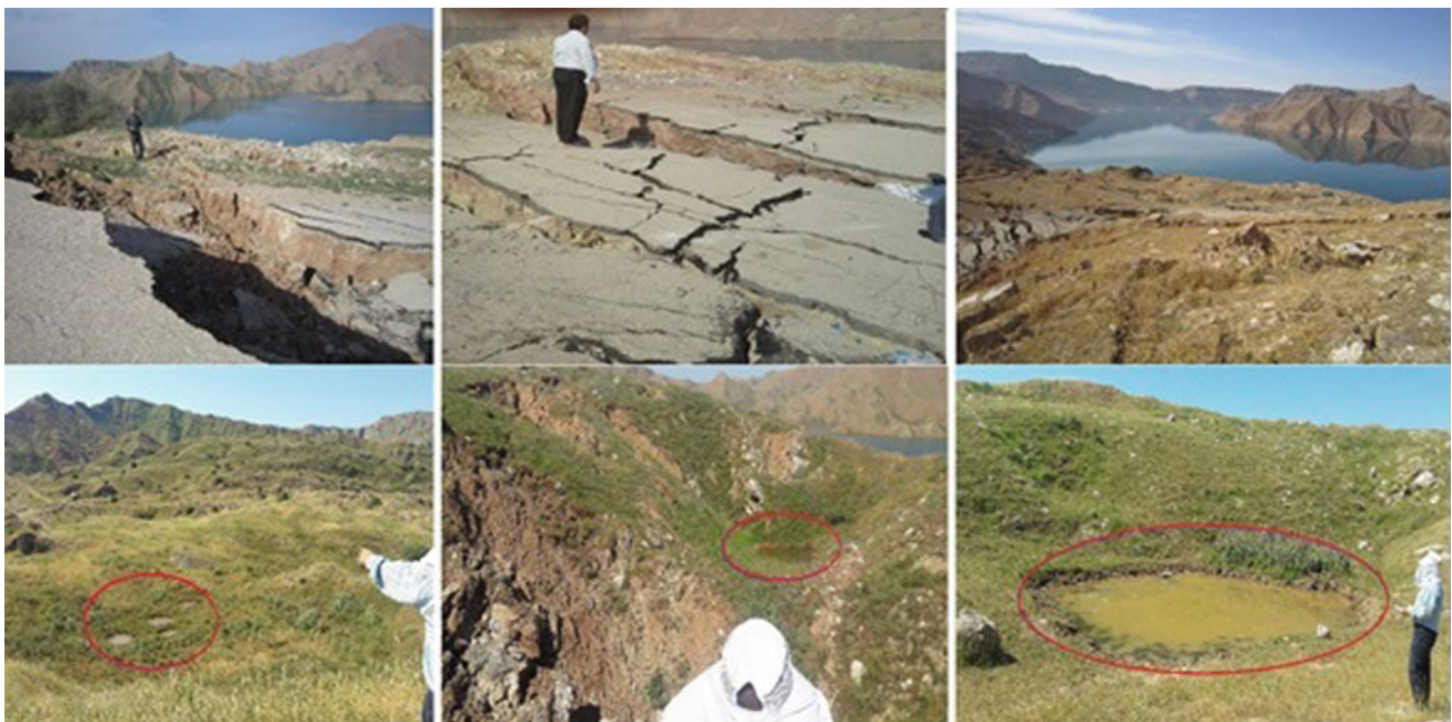
Fig. 7 Progressive sliding and subsidence of the reservoir margin before (top) and after (bottom) the March 2019
