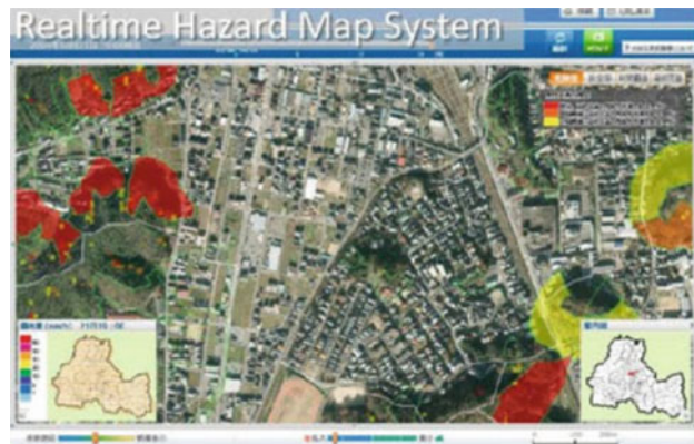
Fig. P.1 Our realtime hazard map reflects up-to-date information of soil natures and precipitations at landslide hazard sites, etc. that can constantly be changing, and evaluates area-wide hazard risk in real-time
